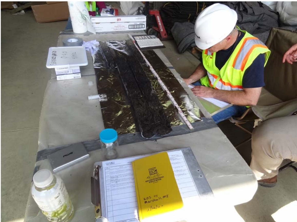
6. RI crews logging soil cores at C3.2 boat launch.
