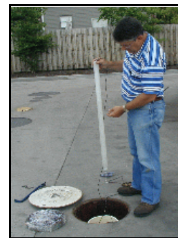
Bailing A Groundwater Monitoring Well
