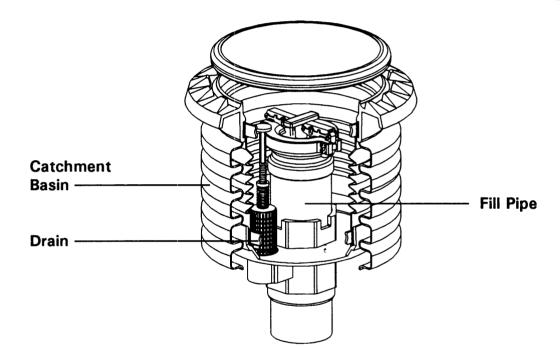
You should try to keep water out of catchment basins. Some catchment basins can collect enough water and sediment, along with spilled product, to make draining this mixture into the tank unwise. If this happens, you may pump out the catchment basin and dispose of the liquid properly. If the liquid contains fuel or chemicals, it could be considered a hazardous waste. Contact your state agency responsible for hazardous waste for information on testing and handling requirements.
