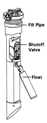
Some automatic shutoff devices work in two stages. The first stage drastically reduces the flow of product to alert the driver that the tank is nearly full. The driver can then close the delivery valve and still have room in the tank for the product left in the delivery hose.
