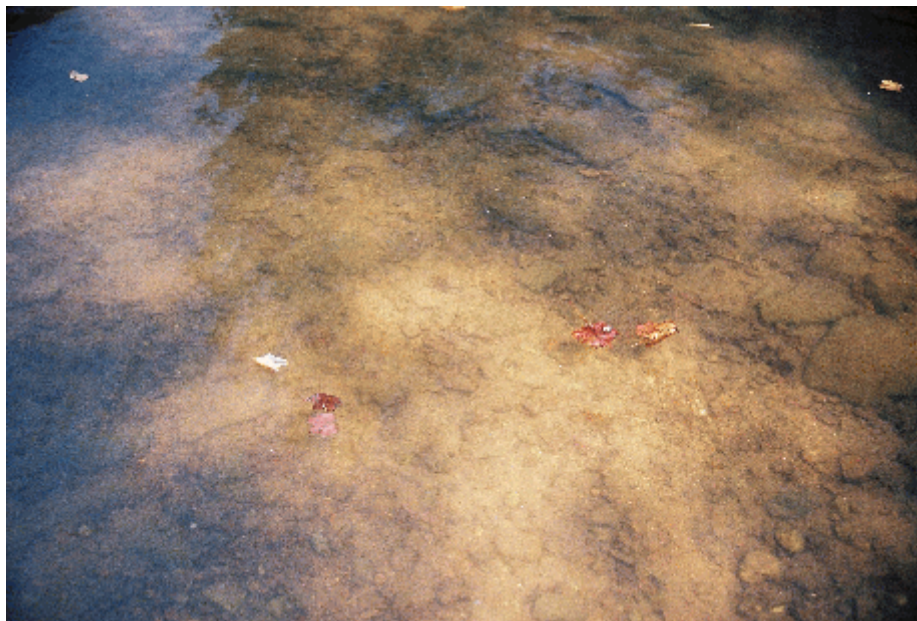
Figure 5. Photograph of the bed surface material at Cahaba River Station CR-AT where a Wolman pebble count was conducted on 09/11/02.
