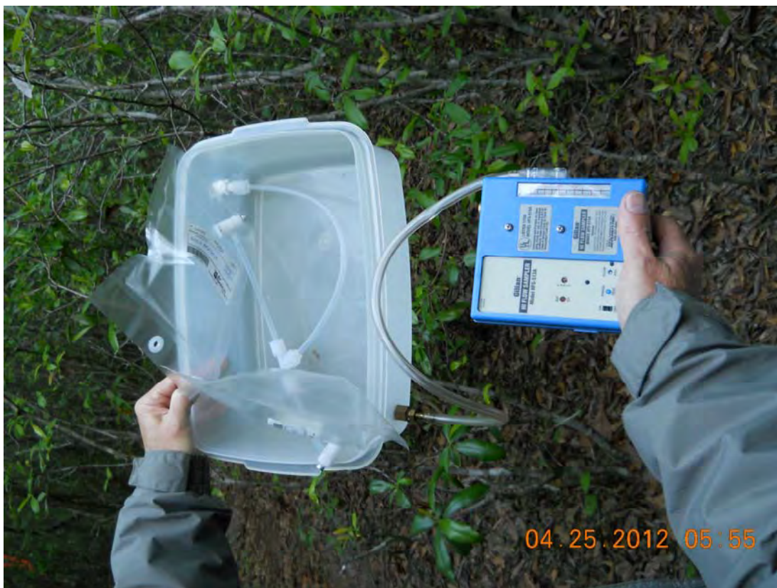
Photo #1 Tedlar Bag Split Sample Collection Apparatus
