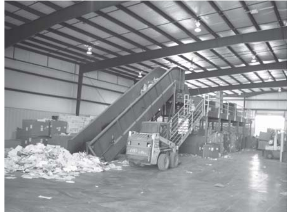
Horizontal balers, like Foothill Sanitation's, are an integral part of many material recovery facilities across the country.
