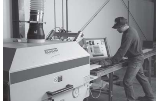
A specialty saw helps refurbish heart pine lumber collected from antique structures across North Carolina slated for demolition.
