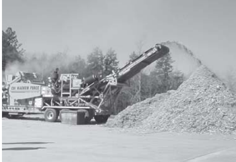
MRR High Point’s wood grinder produces fuel for industrial boilers.
