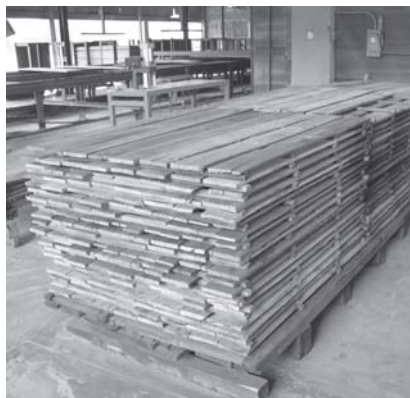
Dismantled pallets are planed into deck boards.
