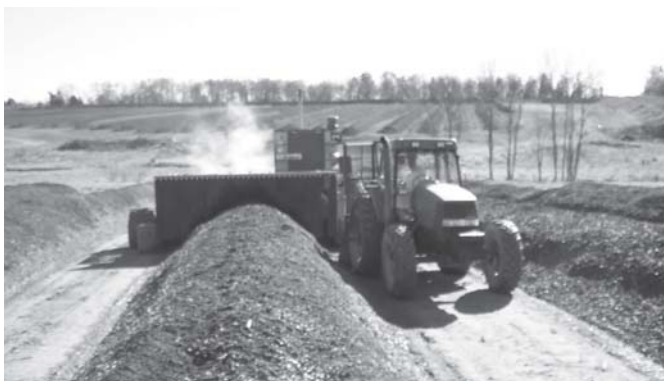
At Wallace Farms, rows of organic debris are turned by a windrow turner to produce high-quality compost.
