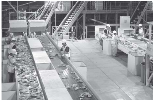
Raleigh RAA employees perform a final manual sort after plastic bottles exit the company's highly automated resin sensors.
