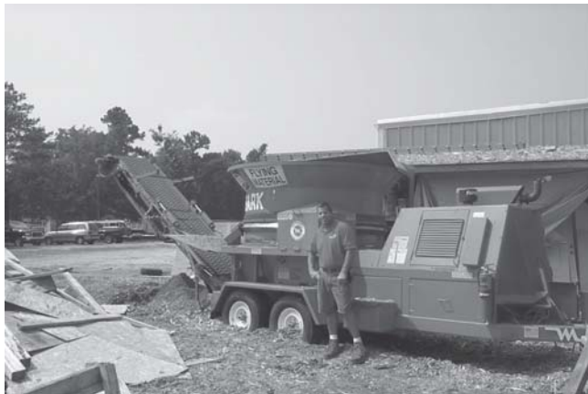
Owner Joe VanEron with the tubgrinder that chips wood debris into mulch and boiler fuel products.
