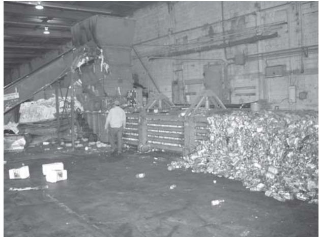
At Bryant's Recycling, plastic bottles are compressed into bales and shipped to market.
