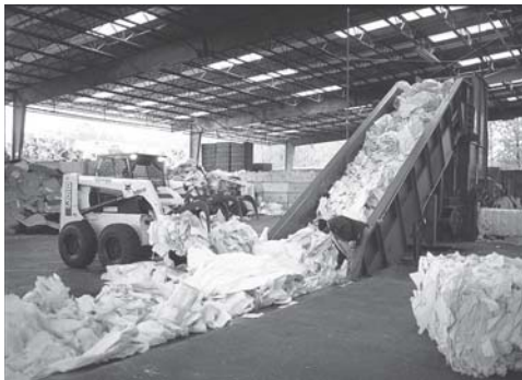
Used paper is inspected and loaded onto a conveyor to be baled and shipped to a paperboard mill.
