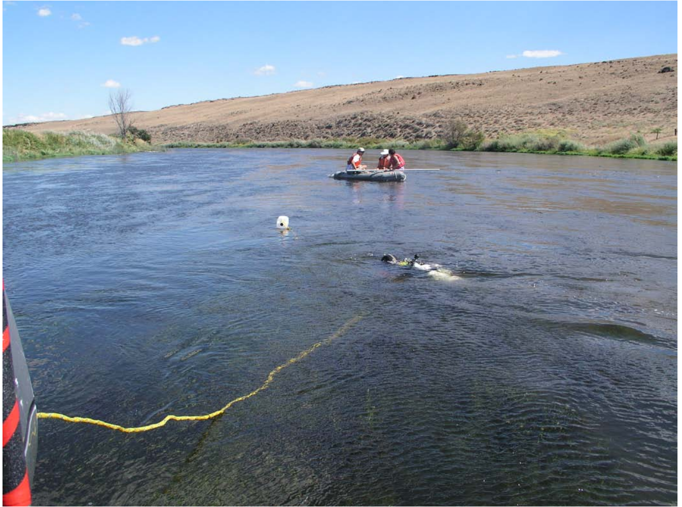
Diver approaches a sampling station on a transect tethered to the boat
