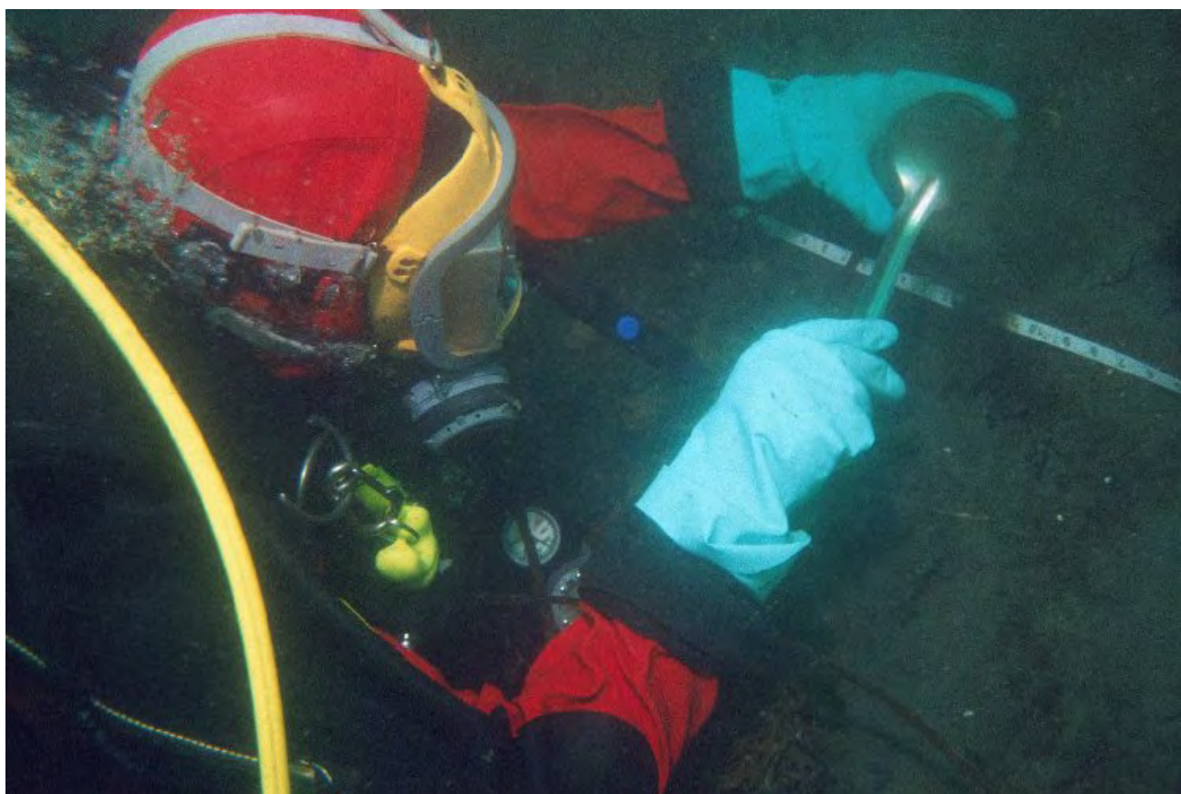
Diver carefully collecting a surface sediment sample.
