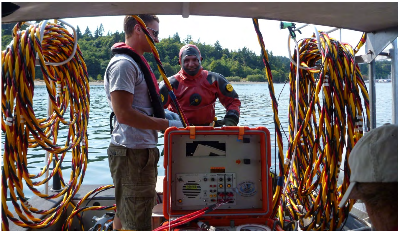
Surface supplied dive equipment was used to search for flux chambers in 2011.
