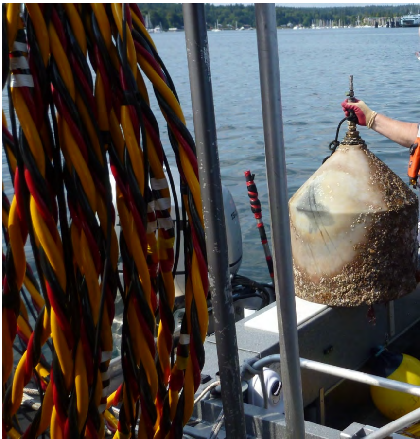
Photo of a flux chamber sampled in 2011, at right.
