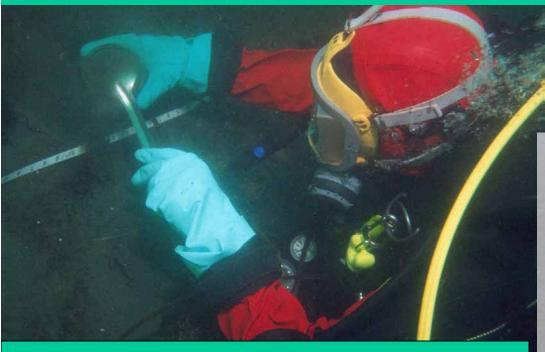
Sampling in a NPDES zone of deposit for a Superfund site groundwater treatment plan outfall.
