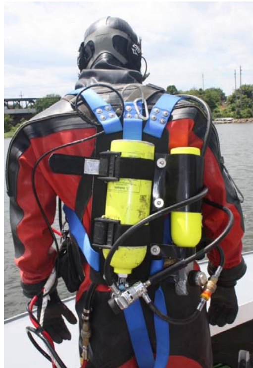
Figure 3. Pony bottle EGS. The smaller tank is an 'accumulation bottle' required for some light weight (e.g., 1/4" air supply hoses) surface-supply systems.
