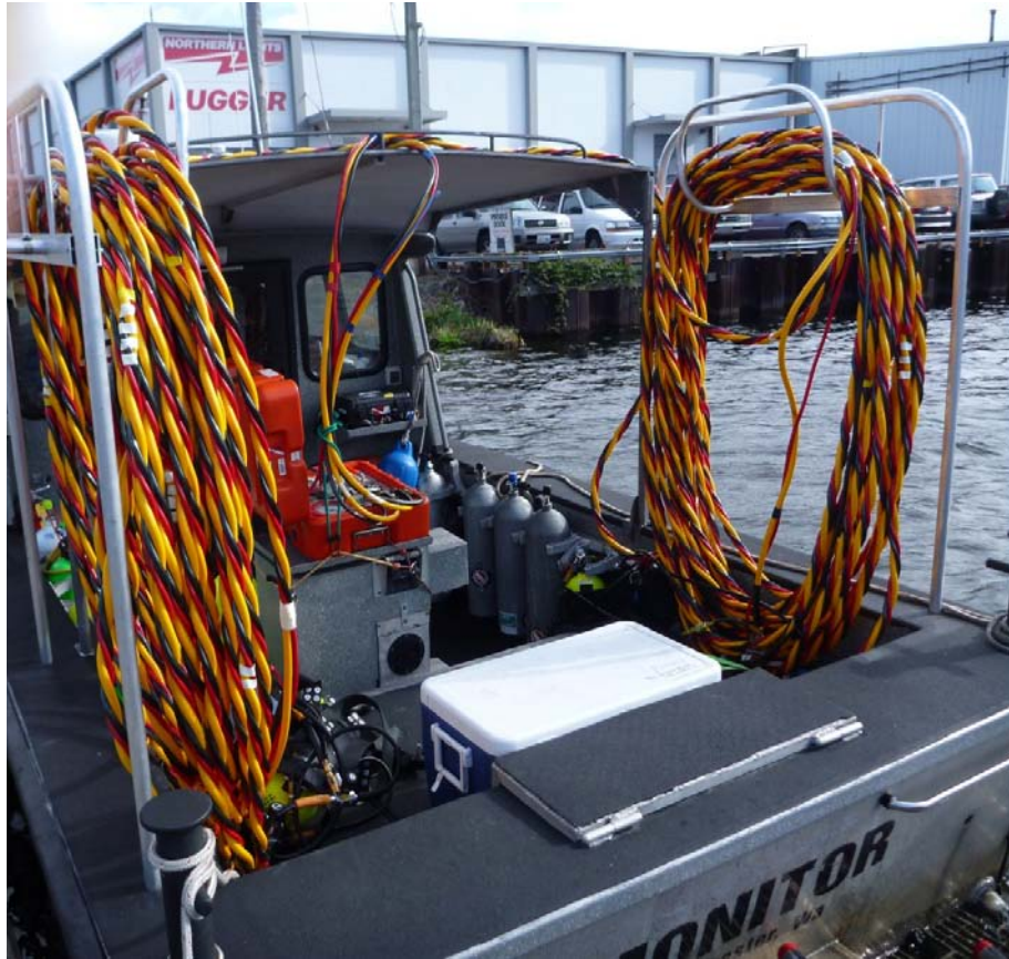
Figure 8. Surface-supply hoses should be managed in the vessel's "hot zone" for polluted water operations.
