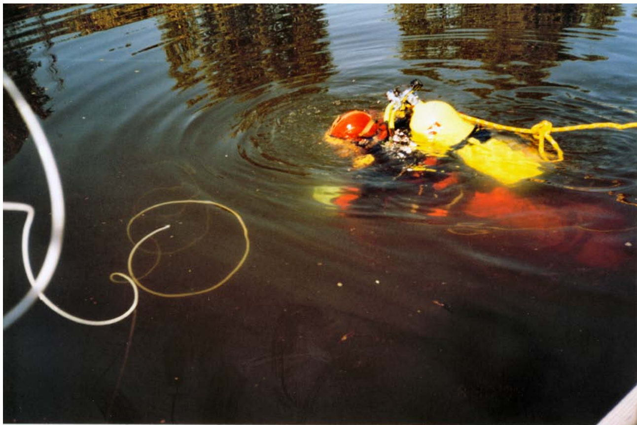
Diver on tether brings piezometer tubing to surface for sample collection
