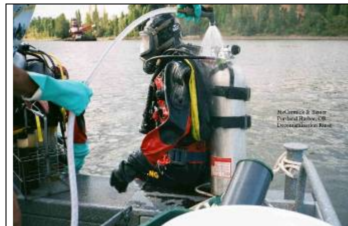
Figure 10: ERT diver undergoing potable water decontamination at the McCormick and Baxter portion of the Portland Harbor Superfund Site. The Region 10 and ERT divers were collecting contaminated bottom sediment cores for lab analysis. Photo by Bruce Duncan, EPA Region 10 Dive Team.
