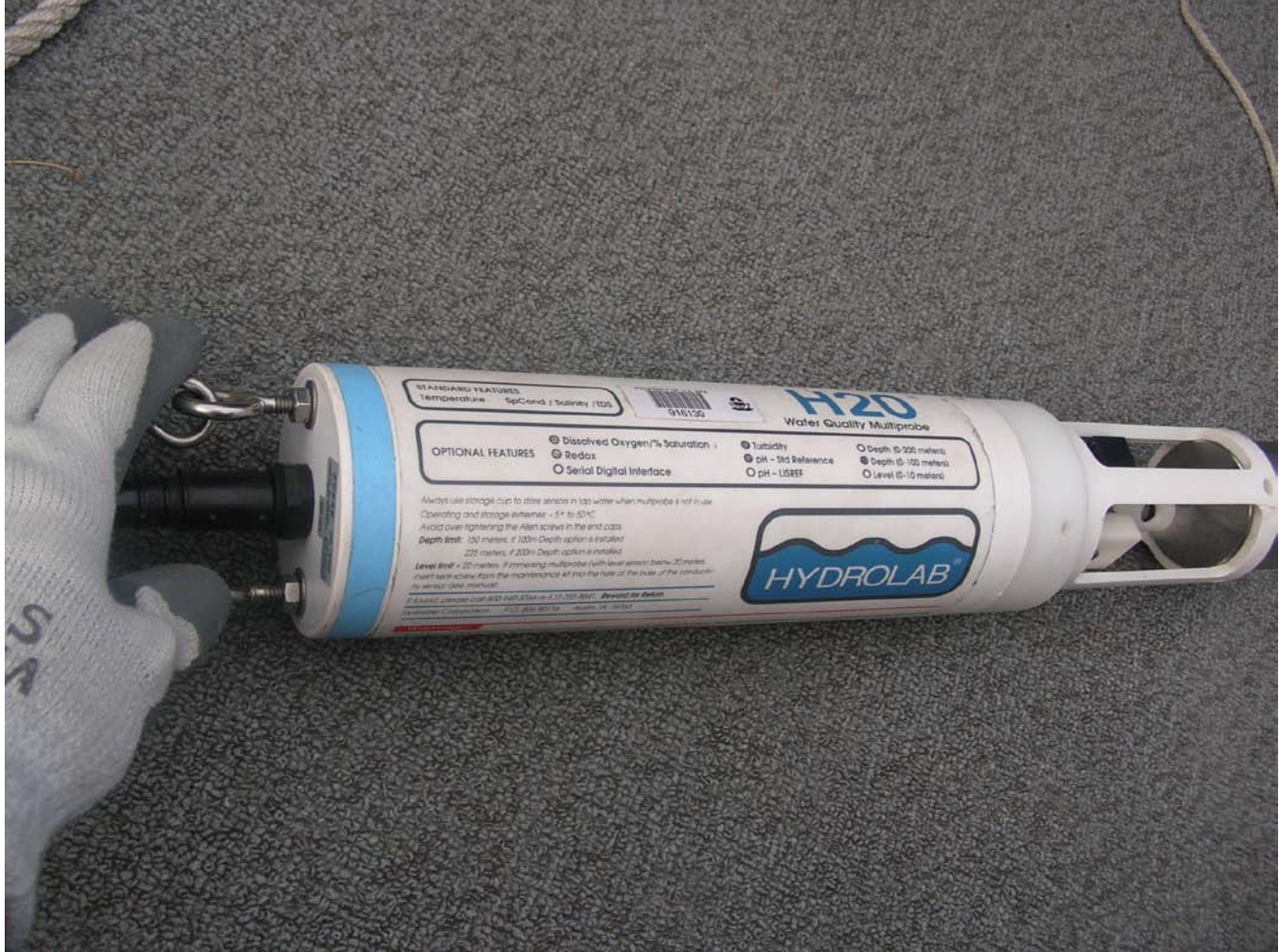
Example data sonde (non functional), used to calibrate the sector scan search and verify the target size could be seen. The actual data sonde lost by WDOE was slightly longer and of a larger diameter.
