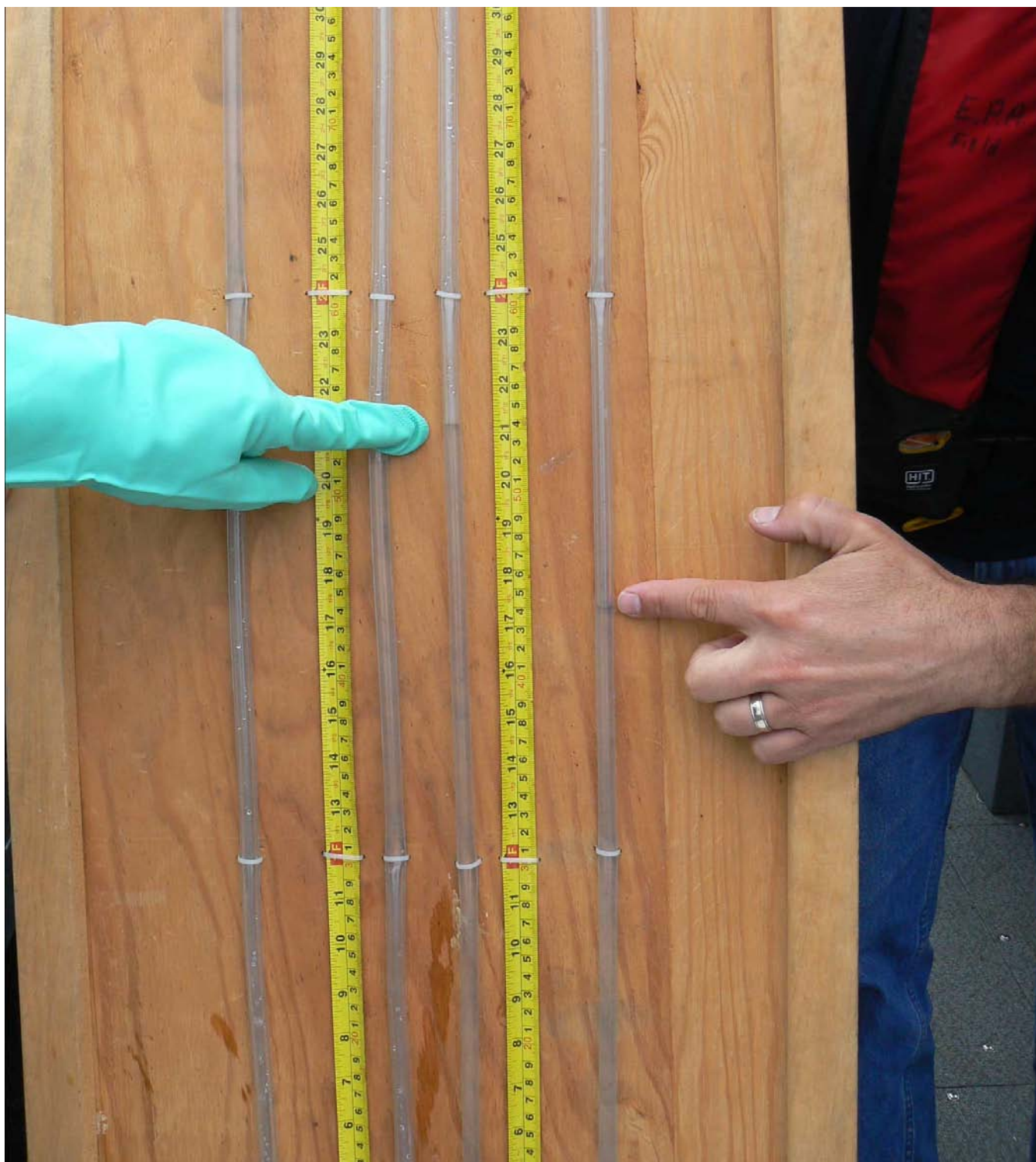
Hydrostatic head between surface water and groundwater being measured by use of a manometer.
