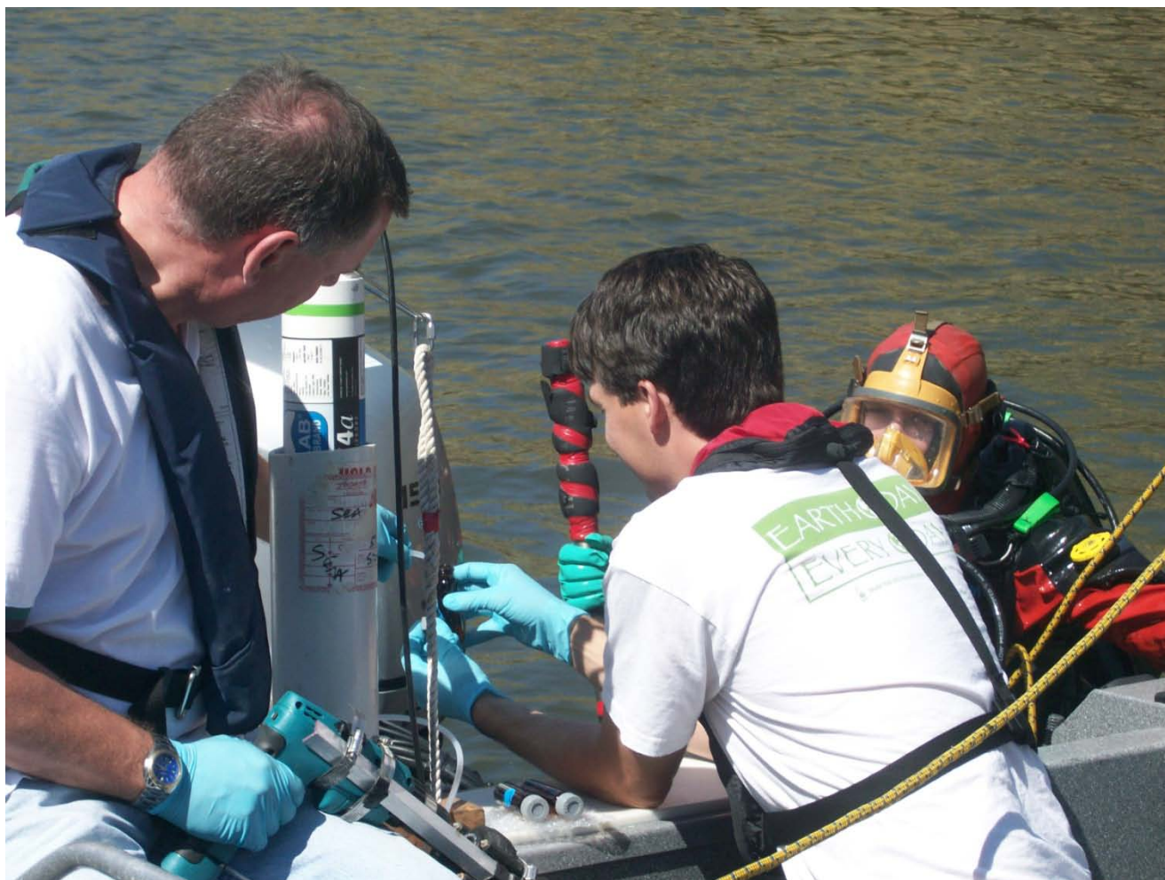
Samplers Curt Black and Brent Richmond collecting groundwater from 50 centimeters into the sediment via piezometers to analyze for chemicals of concern from upland groundwater plumes migrating into the Duwamish River. The diver (Tim Siwiec) that placed the piezometer is in the water in the background, to stay cool due to record heat during 2009 sampling deployments.
