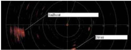
Figure: Screen shot of sector scan images showing the diver and “target” which allows the diver to be directed to the vessel. View of the sector scan sonar, mounted on its tripod (black item on top of grey cylinder on a gimbal), being retrieved.
