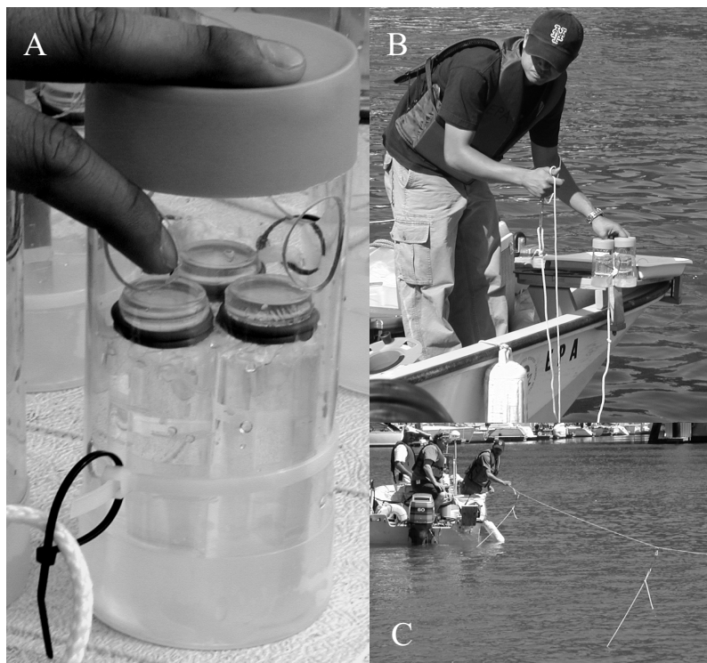
Figure 8. Passive diffusion sampler deployment. A. Triplicate vials within the chamber (chamber is 7.0 cm outside diameter) are covered by a thin polyethylene membrane held in place with two O-rings. (From Duncan et al. , 2007; Fig. 5A. Copyright © 2007 Society of Environmental Toxicology and Chemistry. From Integrated Environmental Assessment and Management . Reprinted by permission of Alliance Communications Group, a division of Allen Press, Inc.). B. Chamber clipped into transect line. C. Deployment of transect line with chambers clipped in.
