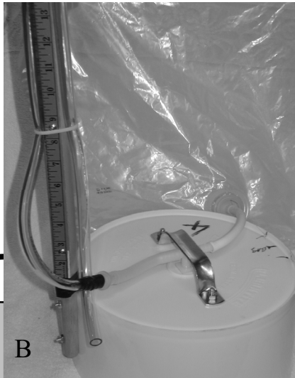
Figure 4. Manometer for measuring hydraulic head. A. Installation by diver: 1. Carry down closed loop with air pocket and place vertically on supporting structure, 2. Disconnect tubing ends, connect one end to piezometer or seepage meter, leave other end open to surface water, read differential head ( \Delta h ) on ruler. B. Mock-up installed on seepage meter. The small bucket seepage meter is an inverted and trimmed 5 gallon (19 L) bucket approximately 26.6 cm outside diameter across the base. C. Example of reading \Delta h on a manometer installed at the surface and connected to a piezometer (left side) and open to the surface water (right side).
