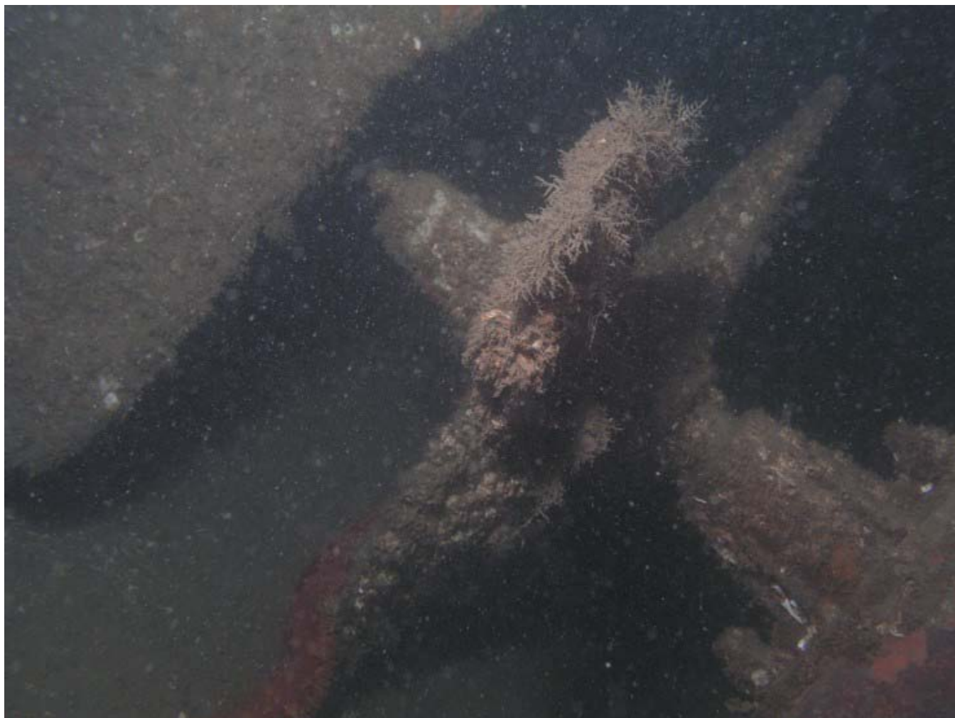
Decaying vessel propeller just above the mudline.
