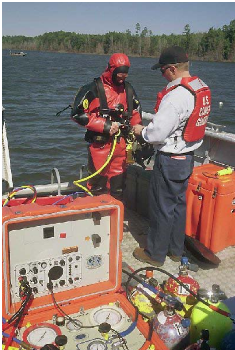
Dan Cooke/ERT prepares Rob Pedersen/UDO/Divemaster/R10 to enter water on surface supplied air.
