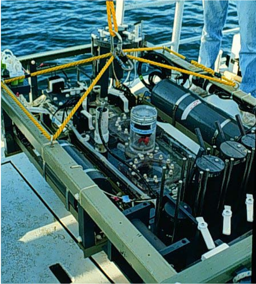
Benthic flux instrument that divers deployed and verified installation of on the Lake bottom.
