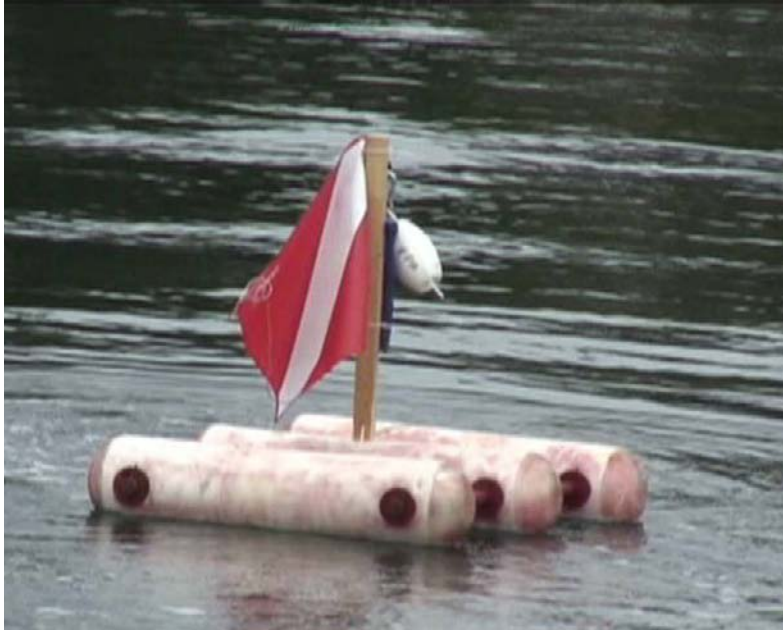
Photo: GPS device carried atop diver towed raft, augmented with a dive flag for safety purposes
