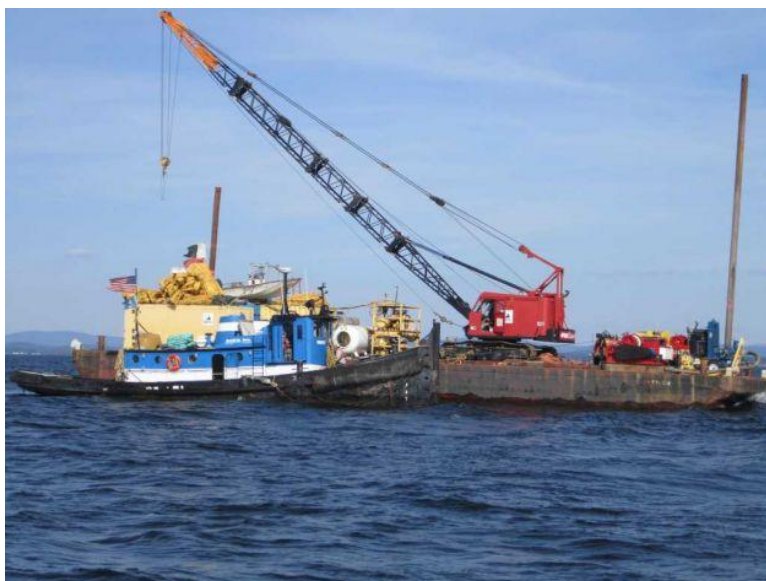
Figure 5: A support tug alongside a diving barge on Lake Champlain, Sept. 21, 2011. Divers explored the wreck of the tugboat, William H. McAllister , that sank decades ago in Lake Champlain to determine if any fuel remains in its tanks. Photo: AP/ AP
