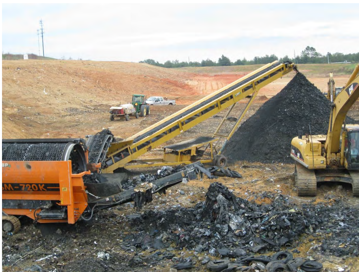
Figure 3-8. View of Screening Waste Materials at a Landfill Reclamation Project in Florida (Photo Courtesy of Innovative Waste Consulting Services, LLC)
