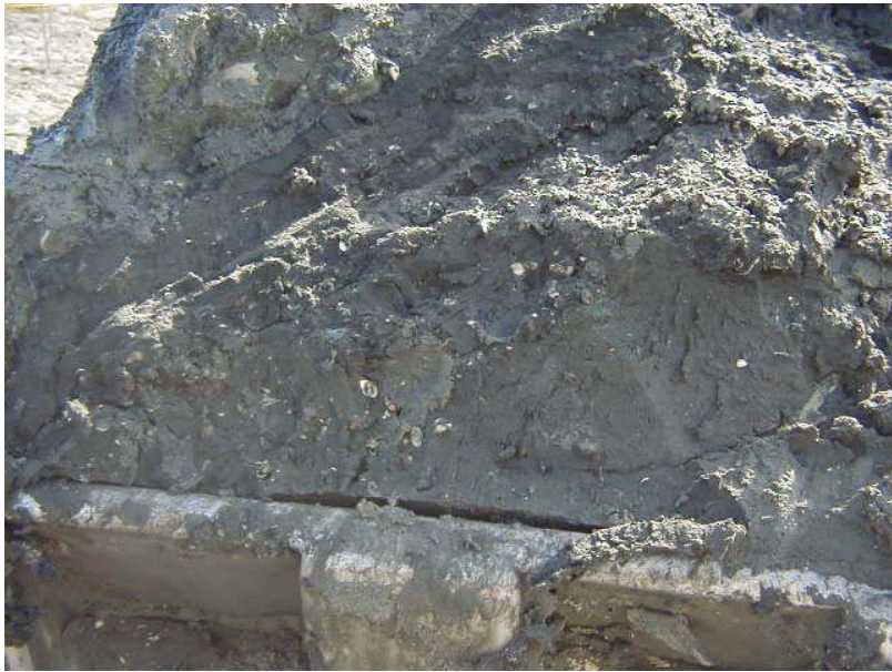
Photo No. 5F: Fill/Organic Clay Interface (TP-D19)
