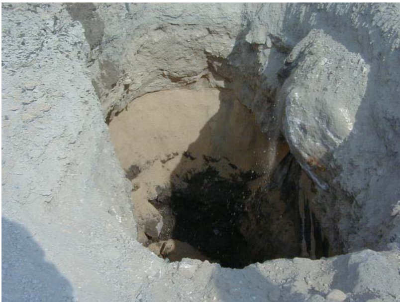
Photo No. 7E: Open Excavation Showing Layering (TP-D10)
