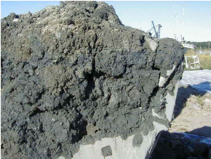
Photo No. 2E: Fill/Organic Clay Interface
