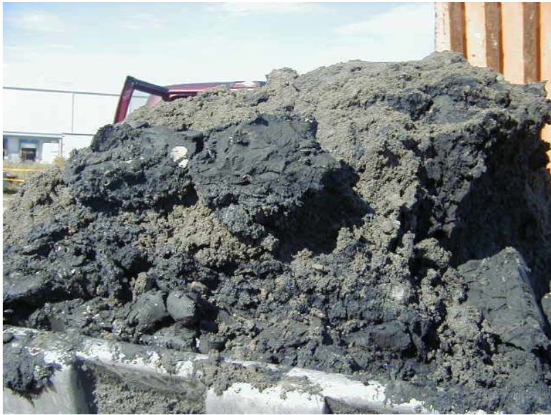
Photo No. 3F: Fill/Organic Clay Interface
