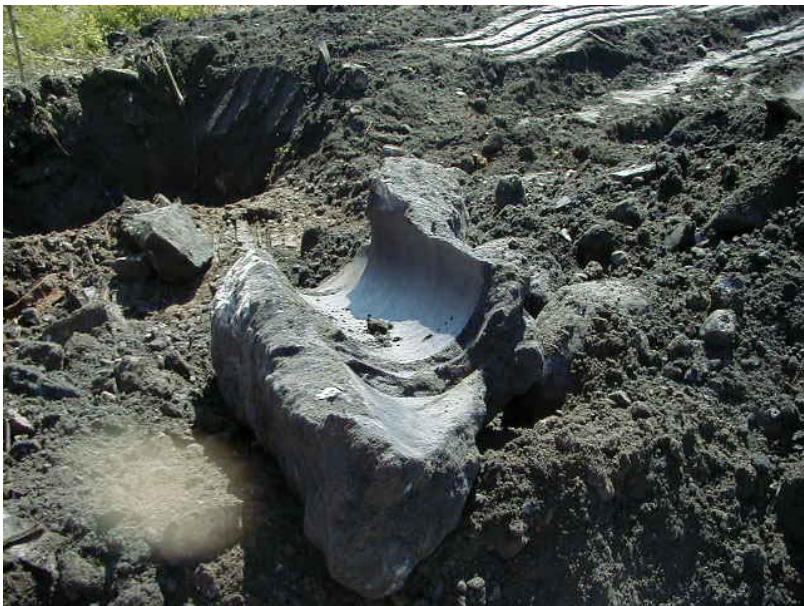
Photo No. 4E: Section of Concrete Encased Pipe (TP-D15)
