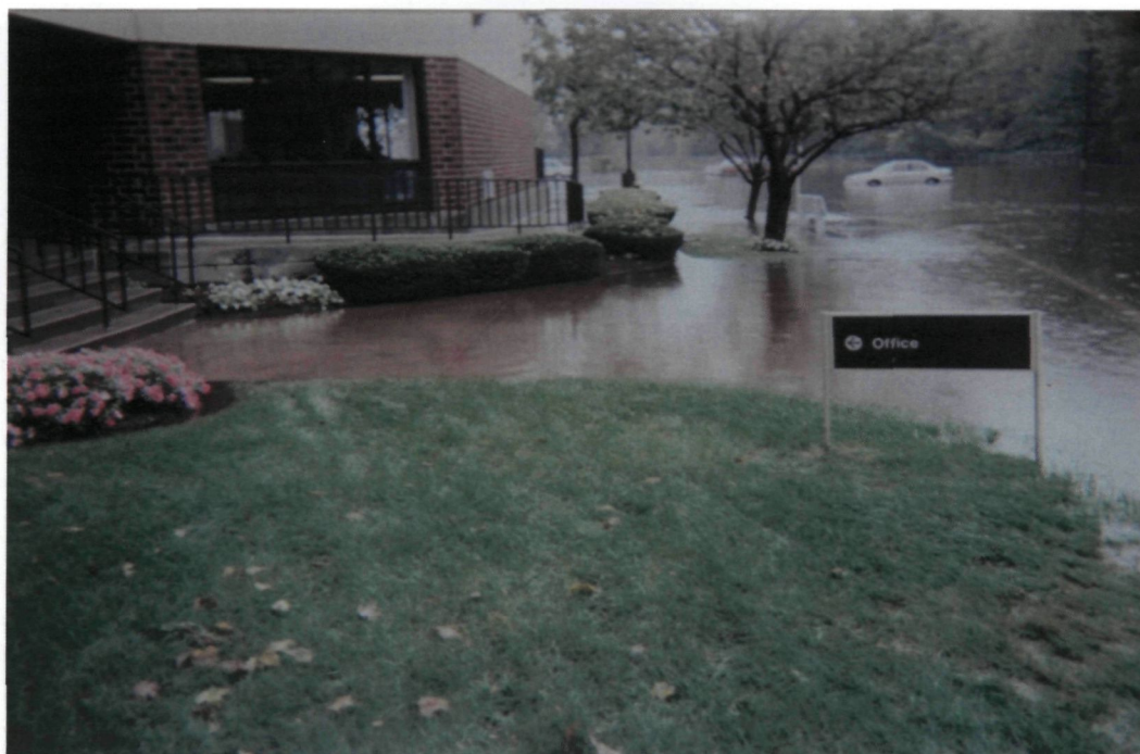
Figure 8. Entrance to Centredale Manor on October 15, 2005. Note that water did not reach the steps to the building; the elevation of the curb near the office sign is approximately 98 ft according to the building as-built plans.
