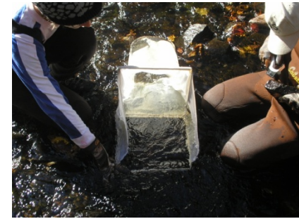
Surber Sampling for Macroinvertebrates • 3 Replicates per riffle (25% Subsamples)
