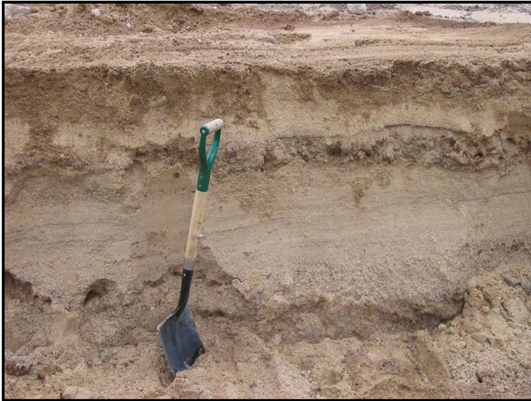
Photograph 3-9 Natural stratification of the soils on the trench sidewall.
