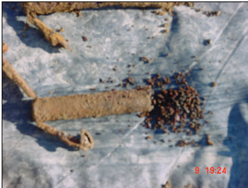
Photograph 7 September 1, 2001 MXU-4/A jet engine starter cartridge igniter assembly recovered in Area A (Item ASP.4.00014), with propellant grain removed
