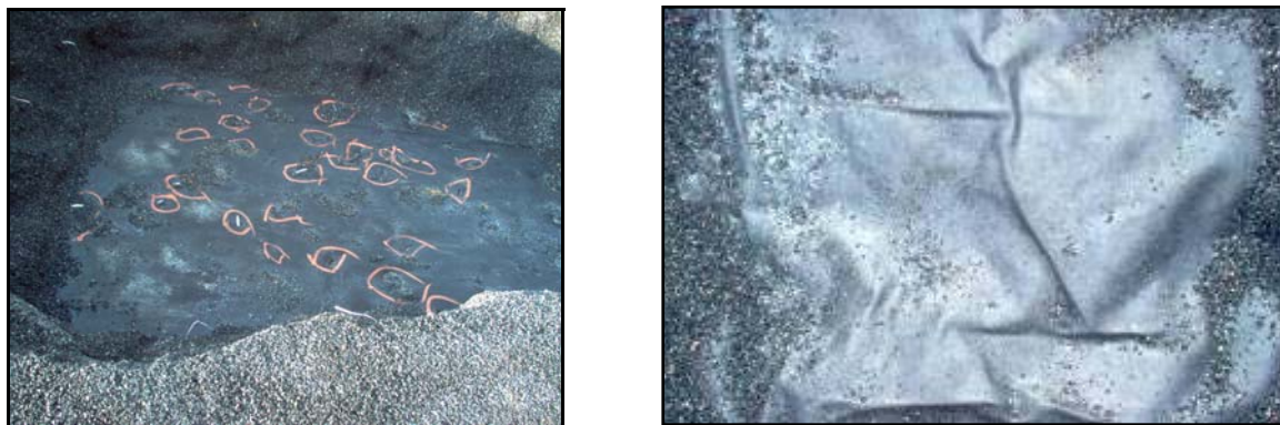
Figure 4-3. Examples of Perforated (left) and Intact (right) Liners (photos not taken at Camp Edwards)
