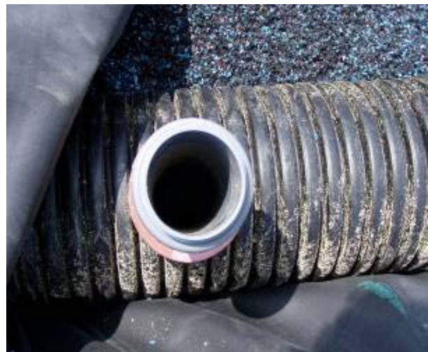
Figure 3-3b. Perforated Pipe & Rubber Granules
