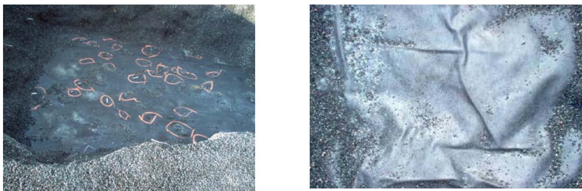
Figure 5-2. Examples of Perforated (left) and Intact (right) Liners (photos not taken at Camp Edwards)
