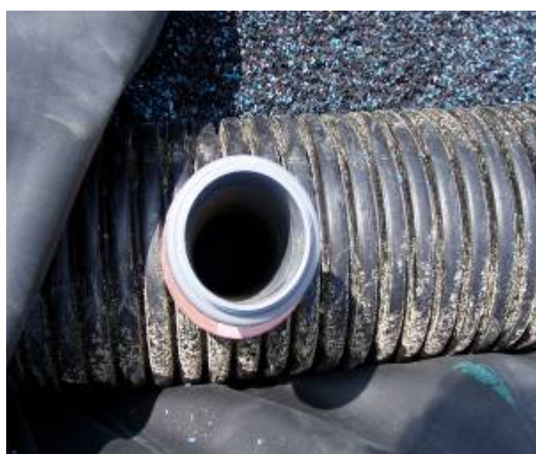
Figure 3-4b Perforated Pipe & Rubber Granules
