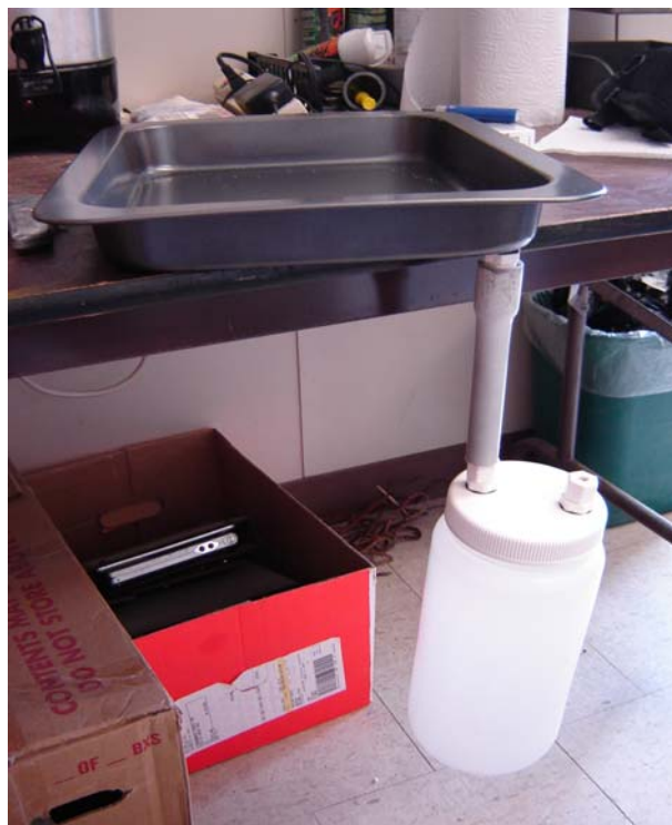
Figure 3-8. Example of a Pan Lysimeter
