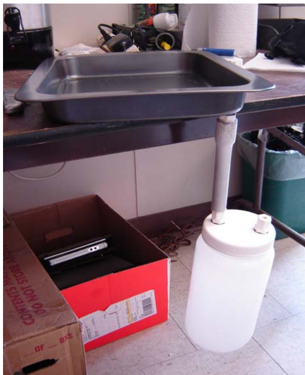
Figure 3-7. Example of a Pan Lysimeter
