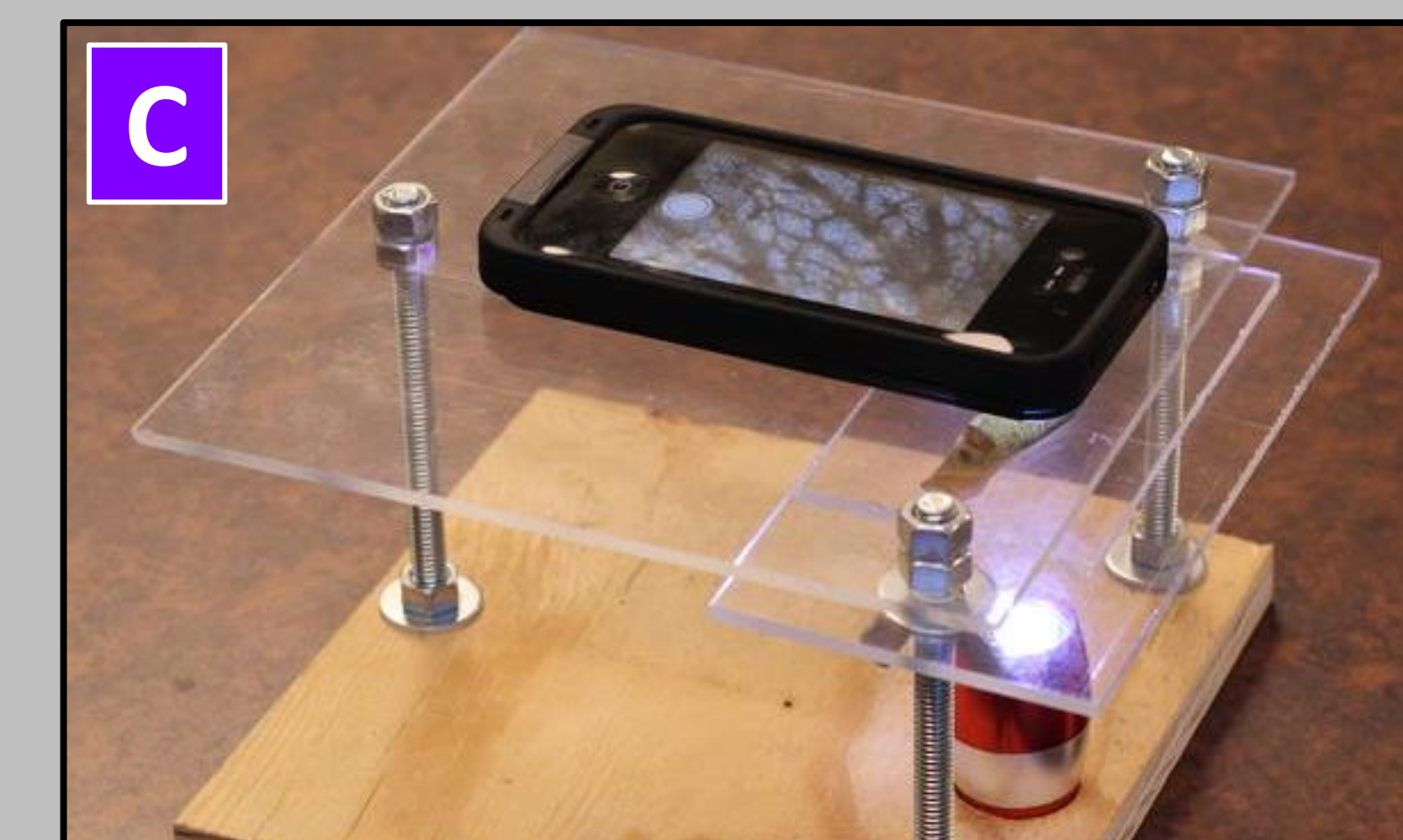
DIY smartphone microscope
