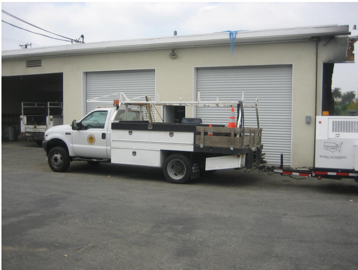
**Figure 5: Utility truck with generator/jet rodder/CCTV trailer**
