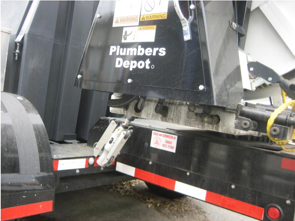
Figure 9: CCTV head on the generator/jet rodder/CCTV trailer
