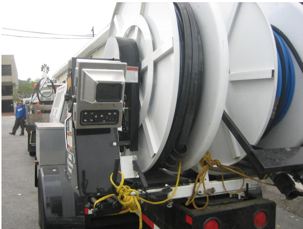
Figure 7: CCTV cable reel on trailer
