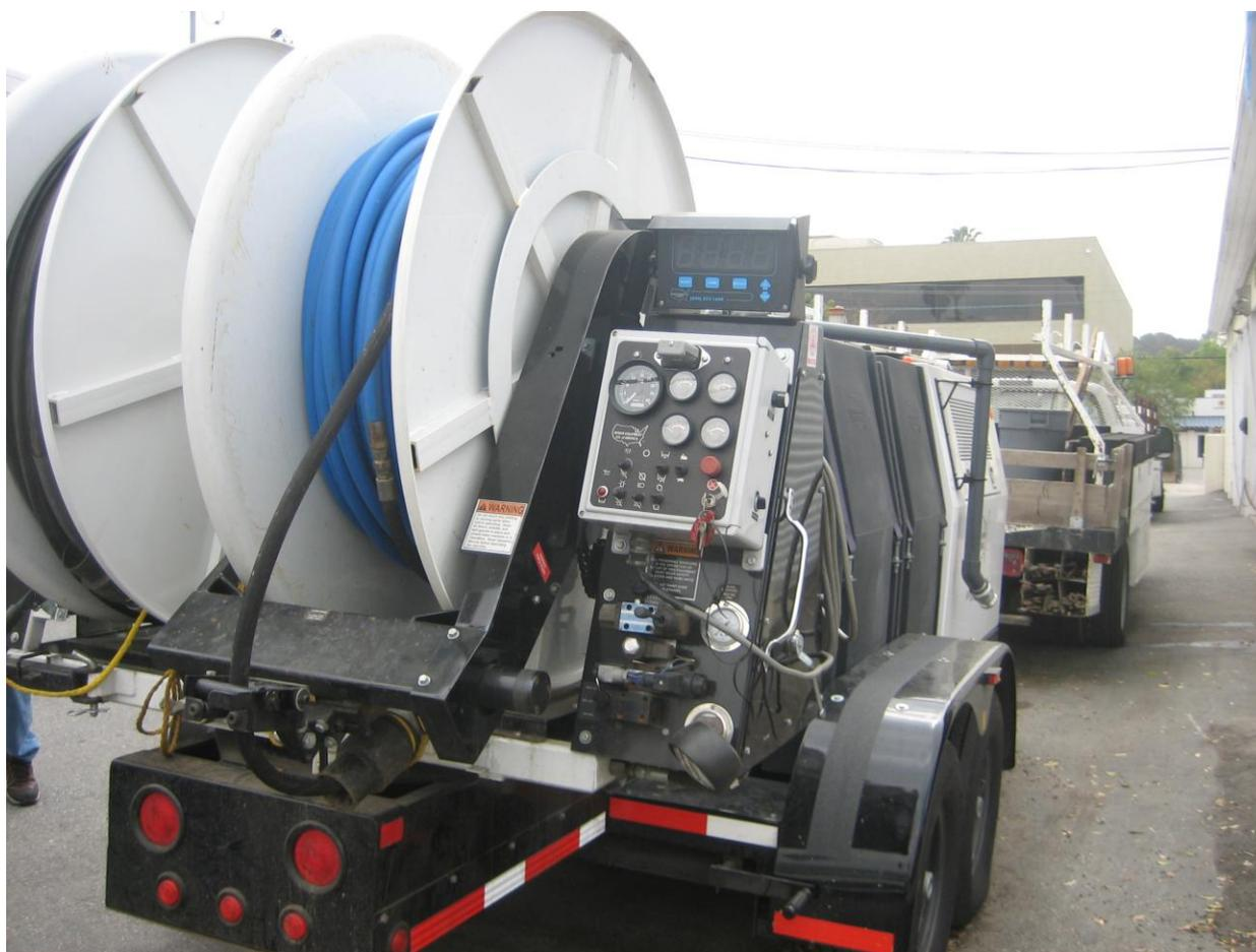
Figure 8: Jet rodder on trailer
