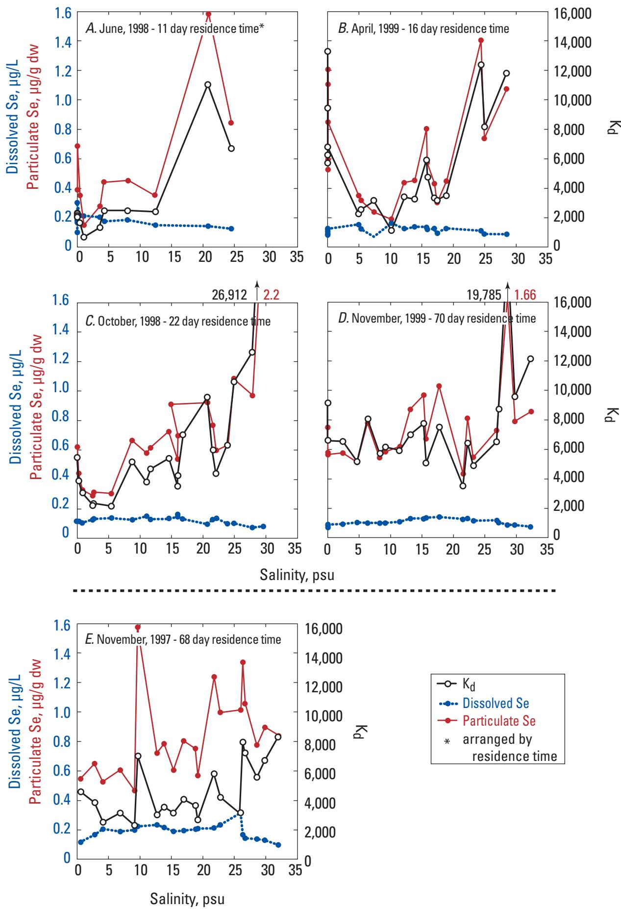
Figure 17. Profiles of observed dissolved and suspended particulate material selenium concentrations and calculated  $K_d$  for transects across the estuary salinity gradient during 1997-1999. [Profiles are arranged in order of increasing residence time, with the profile from November, 1997 separated out (see text for explanation).]
