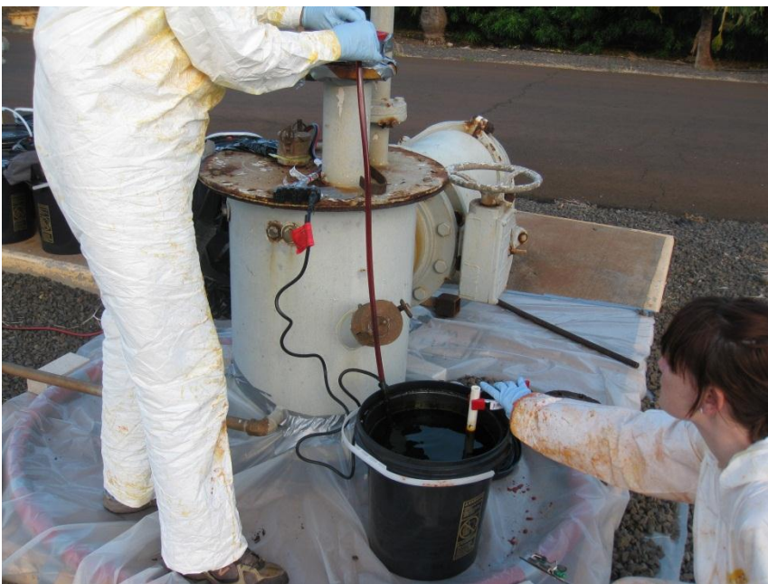
Figure 3-5: Transfer of dye concentrate into injection well 3.
