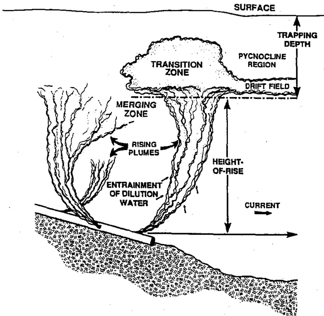
Figure 2. Wastefield generated by a simple ocean outfall (ATSD 1994)
