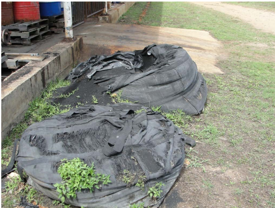
Photo 12: Spilled sandblasting grit was observed on the ground during the inspection.
