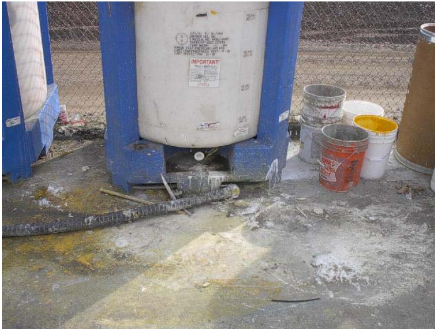
Photo 1: Paint stripping container left open to dry out and drain onto the pavement.
