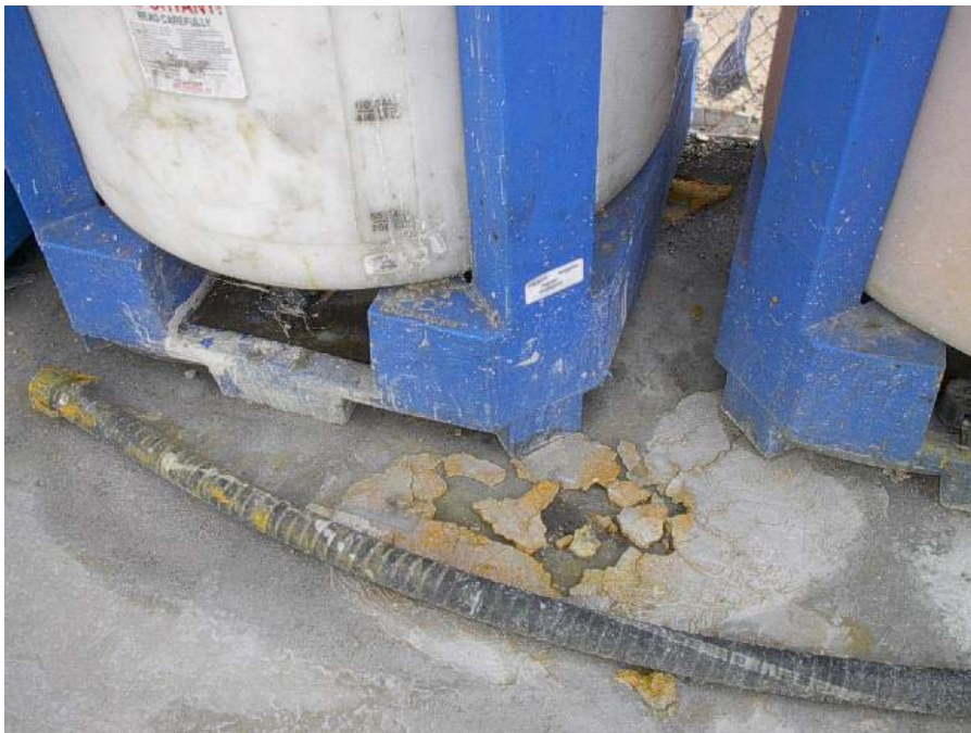
Photo 2: Dry paint on pavement (approximately 1/2 inch thick)
