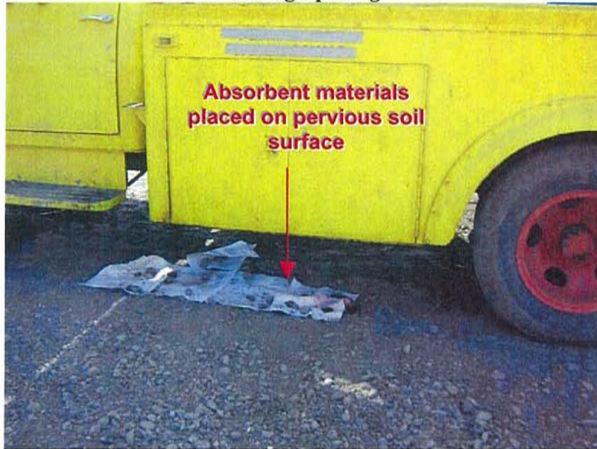
Photograph 9: A mobile fueling truck was actively leaking diesel fuel, and the source of the leak had not been addressed.
