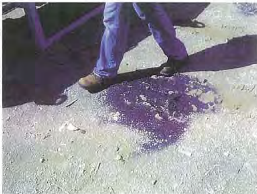
Photo 56: Sand blasting grit was observed on the ground, exposed to potential storm water runoff.
