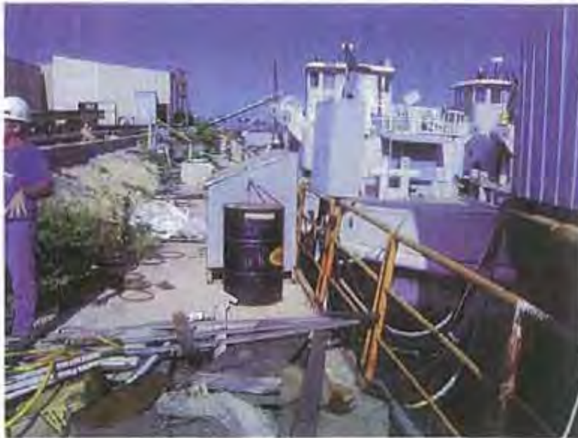
Photo 3: This photograph provides an overview of the dock, beyond the containment berm on the edge of the water, slightly further back than Photo 1. A 55-gallon drum of engine oil was observed on-site, exposed to potential rain fall, adjacent to the receiving water, and without secondary containment.
