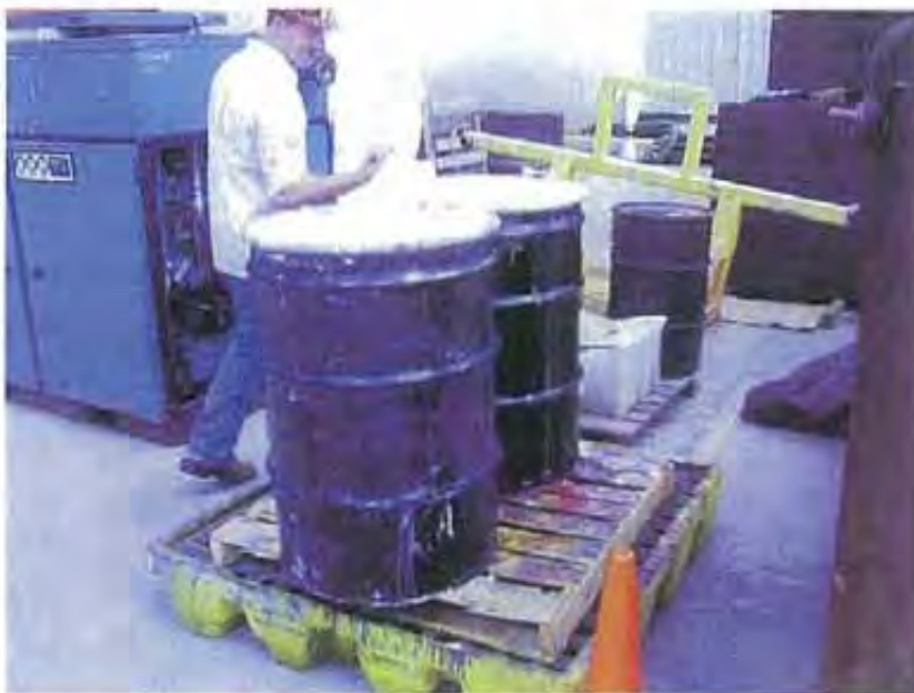
Photo 32: Two 55-gallon drums of "paint related waste" (as described by the Facility representative), which appeared to be a mixture of paint and paint thinner were stored on a secondary containment pallet, in "JR's Area", outside the designated hazardous waste storage area. The drum pictured above was opened by the Discharger at the inspector's request (as shown in Photo 31). One of the drums was hanging over the edge of the containment pallet.
