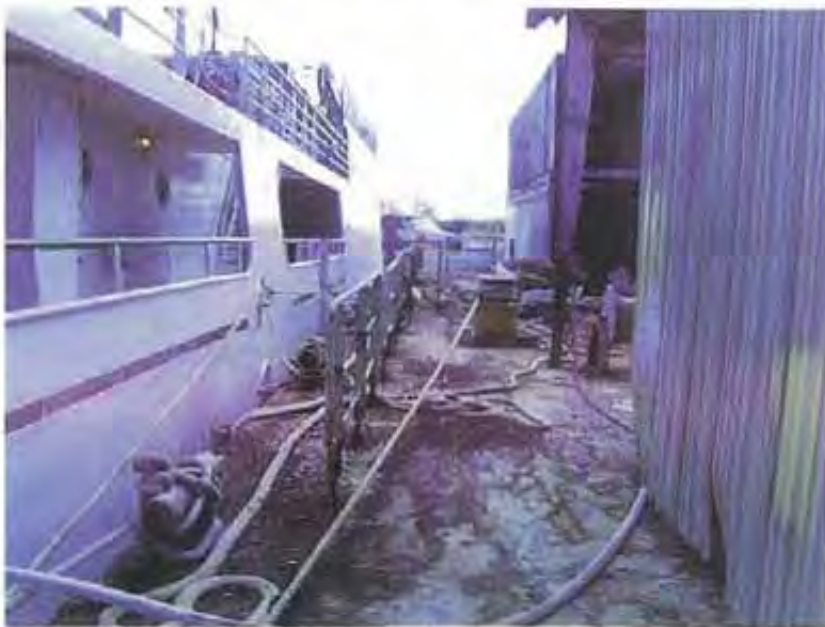
Photo 40: The floor of the work barge was covered in general debris and rust chips/dust, exposed to potential storm water runoff.
