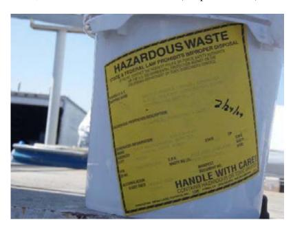
The truck loading area was inspected, included the contents of a truck loaded for transport. Two 55-gallon and two 30-gallon containers of PCB waste were in the truck and were properly labeled. The truck had a PCB label on its outside, as required during transport of PCB waste.
