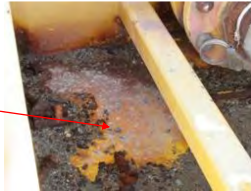
Olympus Stylus 8000, Photo #57; Close-up view of the ground near the valve of the leachate collection frac tank at WMU 34. Note the visible staining.
