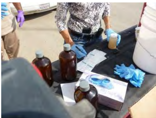
Panasonic Lumix DMC-TZ5, Photo #35; WMU 34 leachate sampling –transferring samples into containers and labeling.
