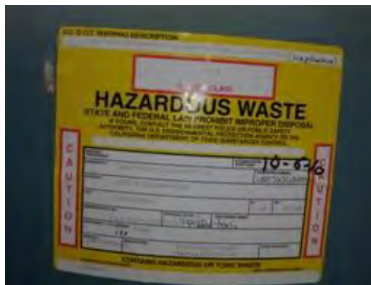
Olympus Stylus 8000, Photo #83; View of the label on a 55-gallon container of F039 leachate (naphthalene) from WMU 33, Cell #3, stored in the less-than-90-day storage area.
