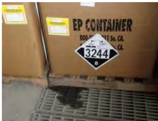
Olympus Stylus 8000, Photo # 16; View of the grate beneath the waste hydrofluoric and sulfuric acid container shown in Photo 15. The liquid on the grate was determined to be rainwater.
