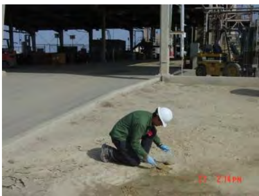
Sony DSC-S75, Photo #22; PCB soil sampling adjacent to the STU access ramp, facing east.
