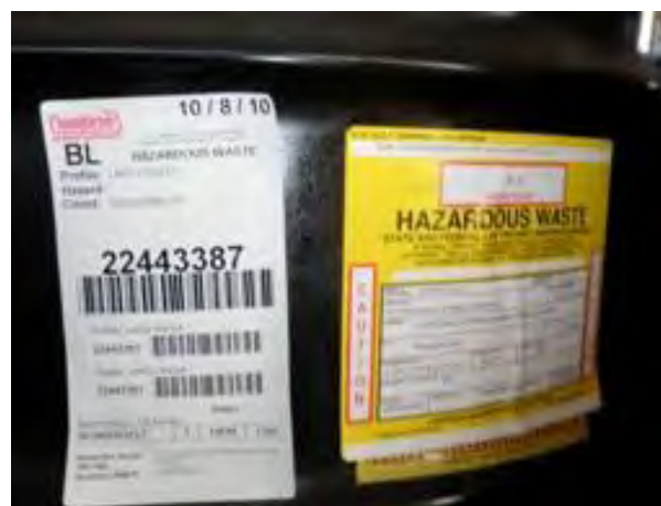
Olympus Stylus 8000, Photo # 13; Close-up view of a label with profile LAP01-9001A (debris with oil) on a 55-gallon container in the drum storage area at DSHA Area 1. This waste is regulated as a California hazardous waste.
