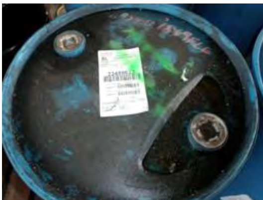
Olympus Stylus 8000, Photo # 26; Drum storage area at the STU, DHS A 5. View of a container of potassium hydroxide waste, received 10/12/10, with oily liquid on top of the lid. No visible leaks or releases.
