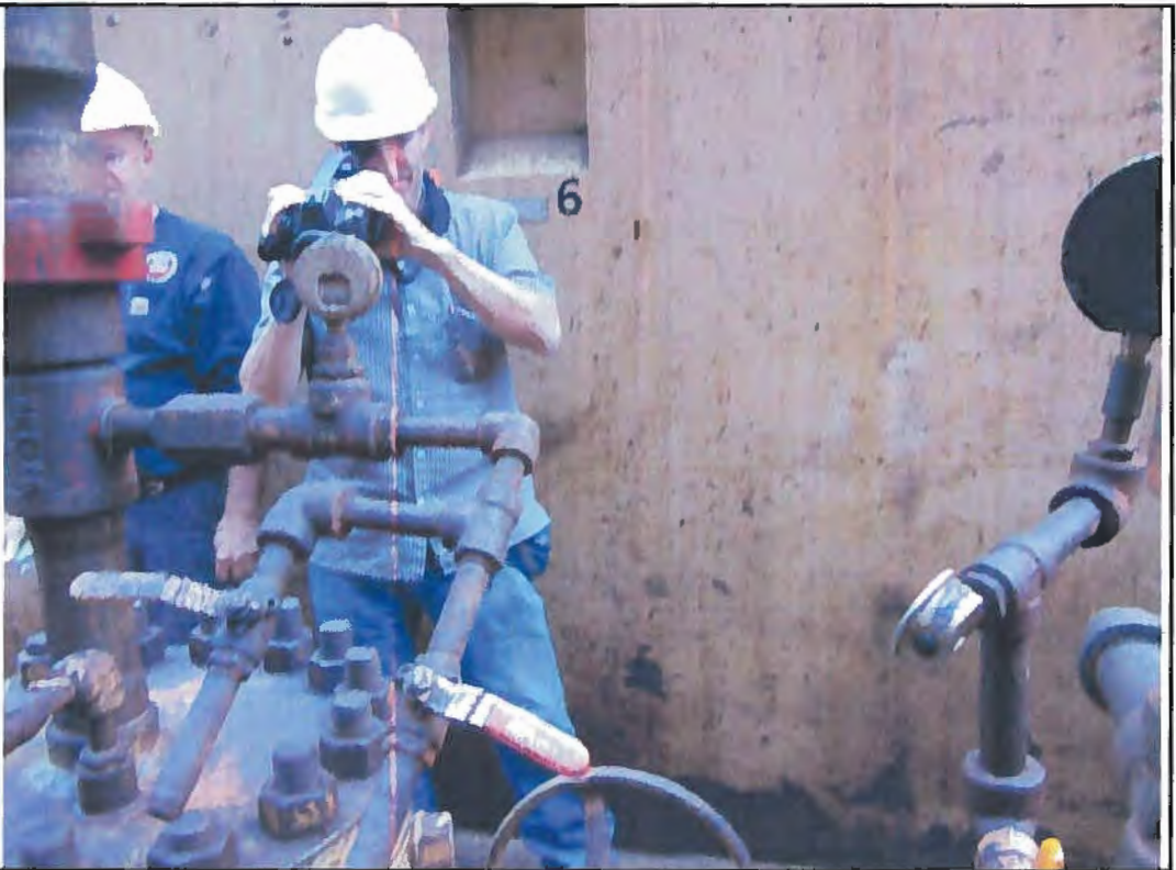
Photo No. 6 Photo Description: Dave Basinger using the FLIR camera at a producing wellhead
