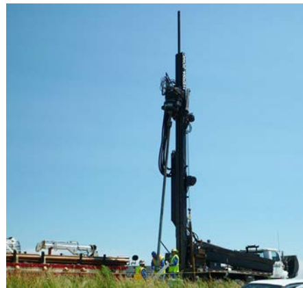
Contractors under EPA oversight perform sonic coring drill sampling at the West Lake Landfill on June 8, 2015. The sampling at the site is being conducted in order to further define locations of radiologically impacted material within the landfill.
