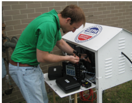
EPA staff checking the operational status of the air monitoring station around the West Lake landfill site.
