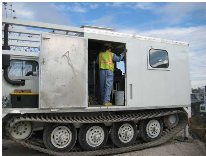
The GCPT direct push rig in action during characterization work at the West Lake Landfill Superfund Site in Bridgeton, Mo., in 2013
