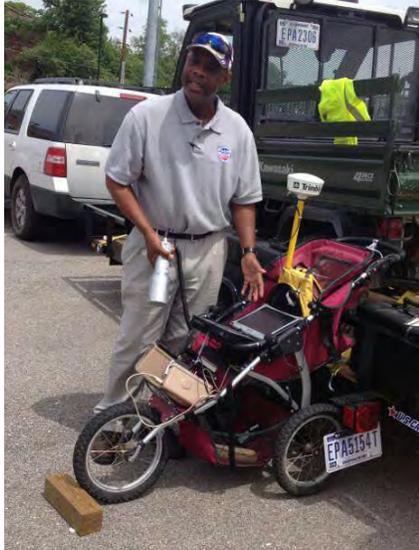
EPA Region 7 is teaming up with EPA Region 5 to conduct the screening using radiation detection instruments, global positioning system equipment, and laptops with software to create mapping products indicating where radiation may be present above natural background levels. The equipment will be mounted on an all-terrain type vehicle or a push cart to maneuver the detectors across the fields in a pattern similar to a grounds keeping crew meticulously mowing Busch Stadium.
