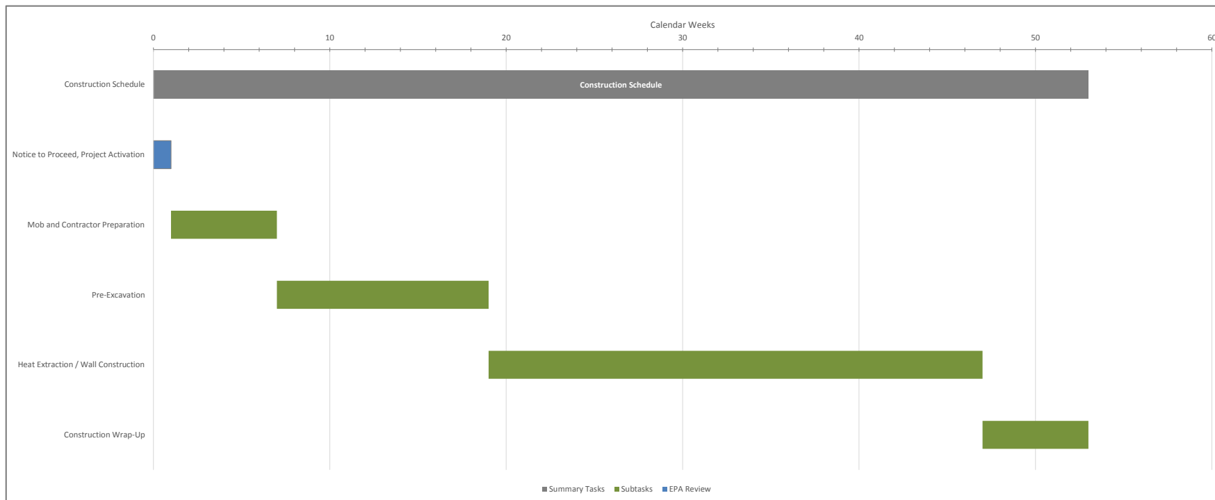
Figure 5 - Estimated Construction Schedule Option 1 (Inert Barrier along Alignment 1)
