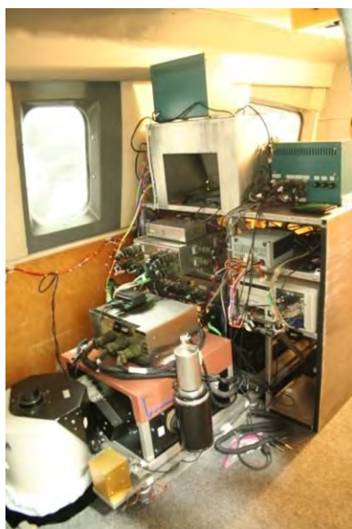
Figure 3 - View of infrared sensors: high speed infrared spectrometer, lower left corner; infrared line scanner is out of view behind the line scanner
