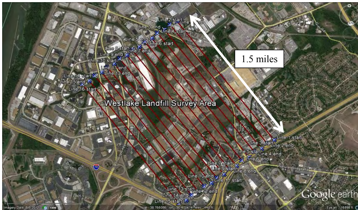
Figure 4: Flight lines radiological survey over West Lake Landfill site.
