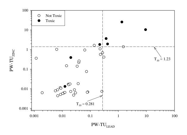
Figure A4-11. Scatter plot showing the relationship between pore-water lead concentrations (PW-TU<sub>LEAD</sub>) and pore-water zinc concentrations (PW-TU<sub>ZINC</sub>), showing samples that were designated as toxic or not toxic based on the survival of midges (*Chironomus dilutus*) in 10-d exposures to sediment samples from the Tri-State Mining District.
