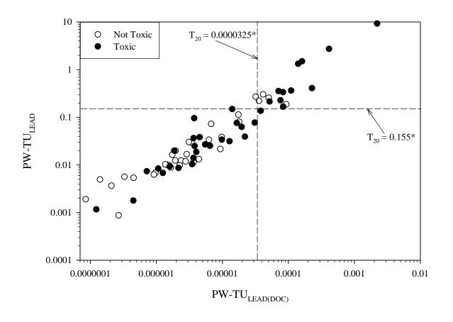
Figure A4-31. Scatter plot showing the relationship between pore-water lead concentrations (PW-TU<sub>LEAD</sub>) and pore-water metal concentrations (ΣPW-TU<sub>DIVALENT METALS</sub>), showing samples that were designated as toxic or not toxic based on the survival of amphipods (*Hyalella azteca*) in 28-d exposures to sediment samples from the Tri-State Mining District.
