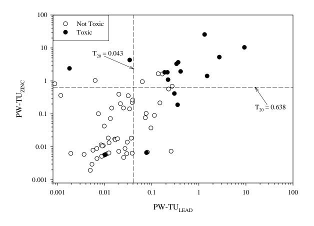
Figure A4-9. Scatter plot showing the relationship between pore-water lead concentrations (PW-TU<sub>LEAD</sub>) and pore-water zinc concentrations (PW-TU<sub>ZINC</sub>), showing samples that were designated as toxic or not toxic based on the survival of mussels (*Lampsilis siliquoidea*) in 28-d exposures to sediment samples from the Tri-State Mining District.
