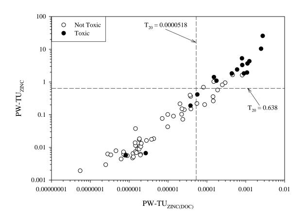
Figure A4-15. Scatter plot showing the relationship between pore-water zinc concentrations normalized to dissolved organic carbon (PW-TU<sub>ZINC(DOC)</sub>) and pore-water zinc concentrations (PW-TU<sub>ZINC</sub>), showing samples that were designated as toxic or not toxic based on the survival of mussels (*Lampsilis siliquoidea*) in 28-d exposures to sediment samples from the Tri-State Mining District.
