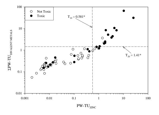
Figure A4-24. Scatter plot showing the relationship between pore-water zinc concentrations (PW-TU<sub>ZINC</sub>) and pore-water metal concentrations (ΣPW-TU<sub>DIVALENT METALS</sub>), showing samples that were designated as toxic or not toxic based on the biomass of midges (*Chironomus dilutus*) in 10-d exposures to sediment samples from the Tri-State Mining District.
