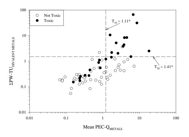
\*Toxicity threshold was derived using 28-d H. azteca toxicity test results (Endpoint: Survival).
