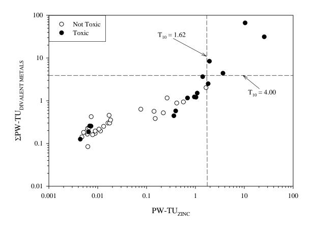
Figure A4-22. Scatter plot showing the relationship between pore-water zinc concentrations (PW-TU<sub>ZINC</sub>) and pore-water metal concentrations (ΣPW-TU<sub>DIVALENT METALS</sub>), showing samples that were designated as toxic or not toxic based on the biomass of mussels (*Lampsilis siliquoidea*) in 28-d exposures to sediment samples from the Tri-State Mining District.
