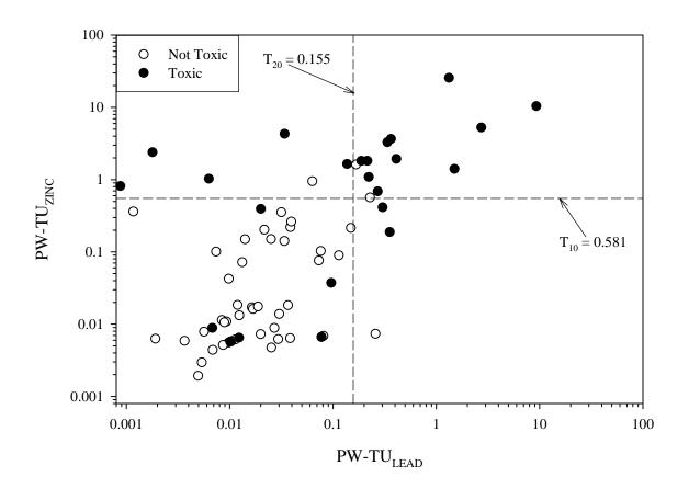
Figure A4-8. Scatter plot showing the relationship between pore-water lead concentrations (PW-TU<sub>LEAD</sub>) and pore-water zinc concentrations (PW-TU<sub>ZINC</sub>), showing samples that were designated as toxic or not toxic based on the biomass of amphipods (*Hyalella azteca*) in 28-d exposures to sediment samples from the Tri-State Mining District.
