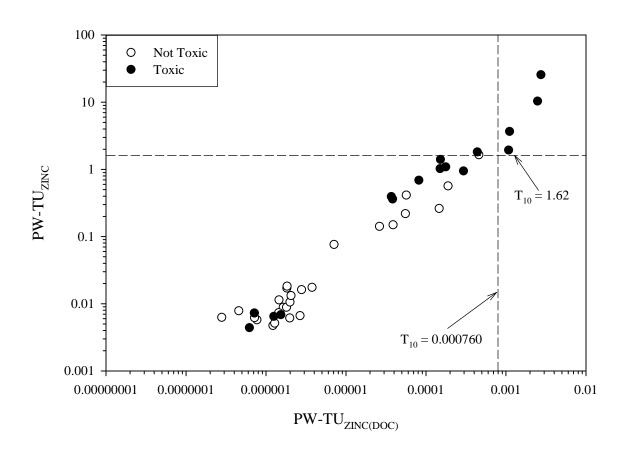
Figure A4-16. Scatter plot showing the relationship between pore-water zinc concentrations normalized to dissolved organic carbon (PW-TU<sub>ZINC(DOC)</sub>) and pore-water zinc concentrations (PW-TU<sub>ZINC</sub>), showing samples that were designated as toxic or not toxic based on the biomass of mussels (*Lampsilis siliquoidea*) in 28-d exposures to sediment samples from the Tri-State Mining District.
