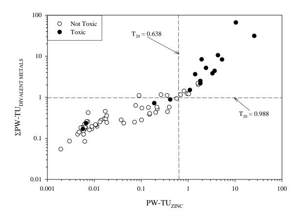
Figure A4-21. Scatter plot showing the relationship between pore-water zinc concentrations (PW-TU<sub>ZINC</sub>) and pore-water metal concentrations (ΣPW-TU<sub>DIVALENT METALS</sub>), showing samples that were designated as toxic or not toxic based on the survival of mussels (*Lampsilis siliquoidea*) in 28-d exposures to sediment samples from the Tri-State Mining District.
