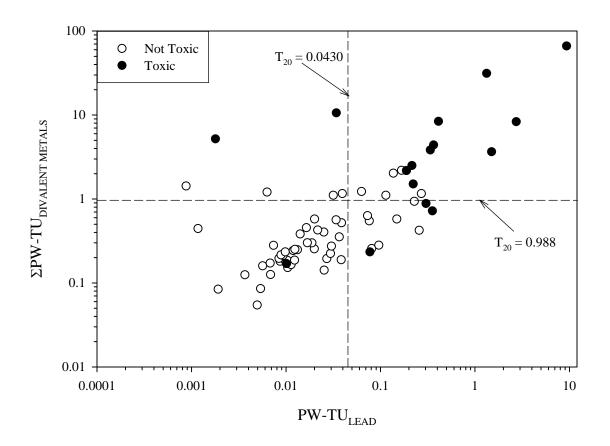
Figure A4-33. Scatter plot showing the relationship between pore-water lead concentrations (PW-TU<sub>LEAD</sub>) and pore-water metal concentrations (ΣPW-TU<sub>DIVALENT METALS</sub>), showing samples that were designated as toxic or not toxic based on the survival of mussels (*Lampsilis siliquoidea*) in 28-d exposures to sediment samples from the Tri-State Mining District.
