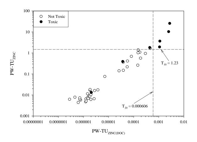
Figure A4-17. Scatter plot showing the relationship between pore-water zinc concentrations normalized to dissolved organic carbon (PW-TU<sub>ZINC(DOC)</sub>) and pore-water zinc concentrations (PW-TU<sub>ZINC</sub>), showing samples that were designated as toxic or not toxic based on the survival of midges (*Chironomus dilutus*) in 10-d exposures to sediment samples from the Tri-State Mining District.
