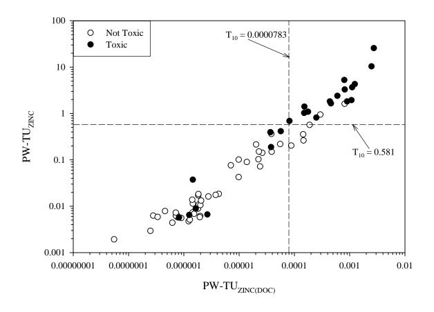
Figure A4-14. Scatter plot showing the relationship between pore-water zinc concentrations normalized to dissolved organic carbon (PW-TU<sub>ZINC(DOC)</sub>) and pore-water zinc concentrations (PW-TU<sub>ZINC</sub>), showing samples that were designated as toxic or not toxic based on the biomass of amphipods (*Hyalella azteca*) in 28-d exposures to sediment samples from the Tri-State Mining District.
