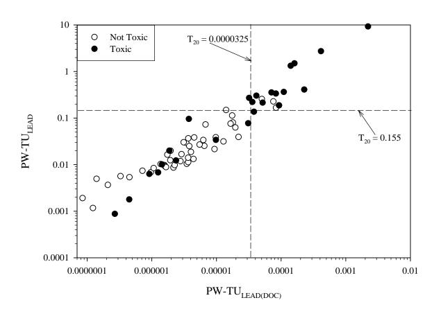
Figure A4-26. Scatter plot showing the relationship between pore-water lead concentrations normalized to dissolved organic carbon (PW-TU<sub>LEAD(DOC)</sub>) and pore-water lead concentrations (PW-TU<sub>LEAD</sub>), showing samples that were designated as toxic or not toxic based on the biomass of amphipods (*Hyalella azteca*) in 28-d exposures to sediment samples from the Tri-State Mining District.
