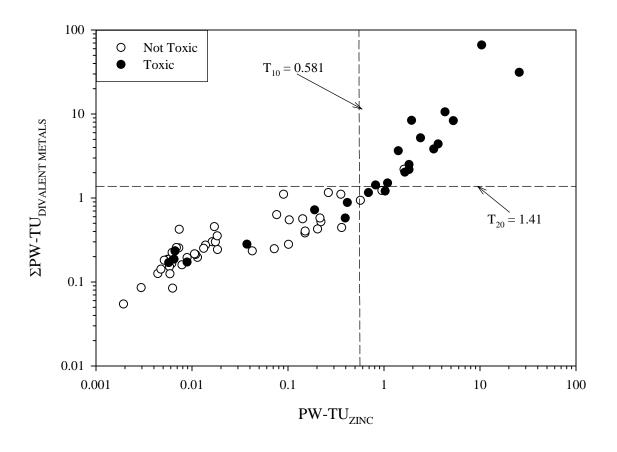
Figure A4-20. Scatter plot showing the relationship between pore-water zinc concentrations (PW-TU<sub>ZINC</sub>) and pore-water metal concentrations (ΣPW-TU<sub>DIVALENT METALS</sub>), showing samples that were designated as toxic or not toxic based on the biomass of amphipods (*Hyalella azteca*) in 28-d exposures to sediment samples from the Tri-State Mining District.
