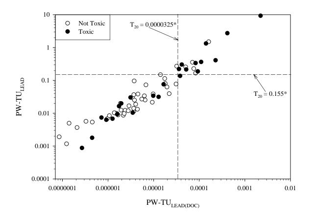
Figure A4-30. Scatter plot showing the relationship between pore-water lead concentrations normalized to dissolved organic carbon (PW-TU<sub>LEAD(DOC)</sub>) and pore-water lead concentrations (PW-TU<sub>LEAD</sub>), showing samples that were designated as toxic or not toxic based on the biomass of midges (*Chironomus dilutus*) in 10-d exposures to sediment samples from the Tri-State Mining District.
