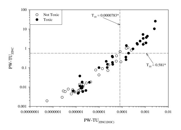
Figure A4-19. Scatter plot showing the relationship between pore-water zinc concentrations (PW-TU<sub>ZINC</sub>) and pore-water metal concentrations (ΣPW-TU<sub>DIVALENT METALS</sub>), showing samples that were designated as toxic or not toxic based on the survival of amphipods (*Hyalella azteca*) in 28-d exposures to sediment samples from the Tri-State Mining District.
