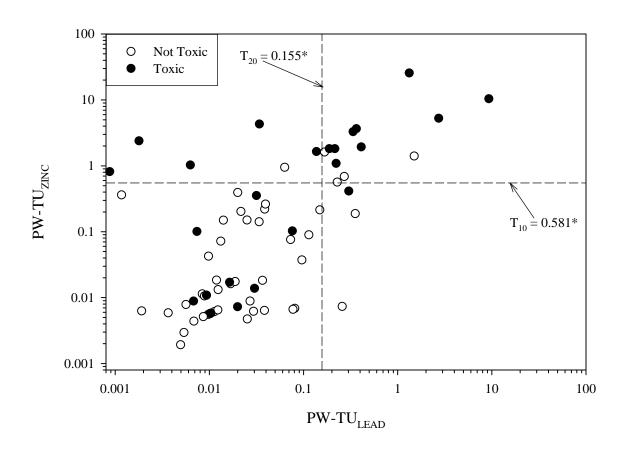
\*Toxicity threshold was derived using 28-d H. azteca toxicity test results (Endpoint: Survival).
