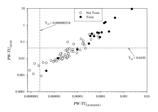
Figure A4-27. Scatter plot showing the relationship between pore-water lead concentrations normalized to dissolved organic carbon (PW-TU<sub>LEAD(DOC)</sub>) and pore-water lead concentrations (PW-TU<sub>LEAD</sub>), showing samples that were designated as toxic or not toxic based on the survival of mussels (*Lampsilis siliquoidea*) in 28-d exposures to sediment samples from the Tri-State Mining District.
