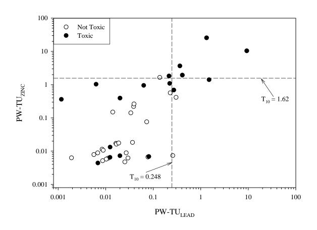
Figure A4-10. Scatter plot showing the relationship between pore-water lead concentrations (PW-TU<sub>LEAD</sub>) and pore-water zinc concentrations (PW-TU<sub>ZINC</sub>), showing samples that were designated as toxic or not toxic based on the biomass of mussels (*Lampsilis siliquoidea*) in 28-d exposures to sediment samples from the Tri-State Mining District.
