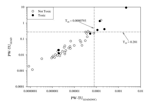
Figure A4-29. Scatter plot showing the relationship between pore-water lead concentrations normalized to dissolved organic carbon (PW-TU<sub>LEAD(DOC)</sub>) and pore-water lead concentrations (PW-TU<sub>LEAD</sub>), showing samples that were designated as toxic or not toxic based on the survival of midges (*Chironomus dilutus*) in 10-d exposures to sediment samples from the Tri-State Mining District.
