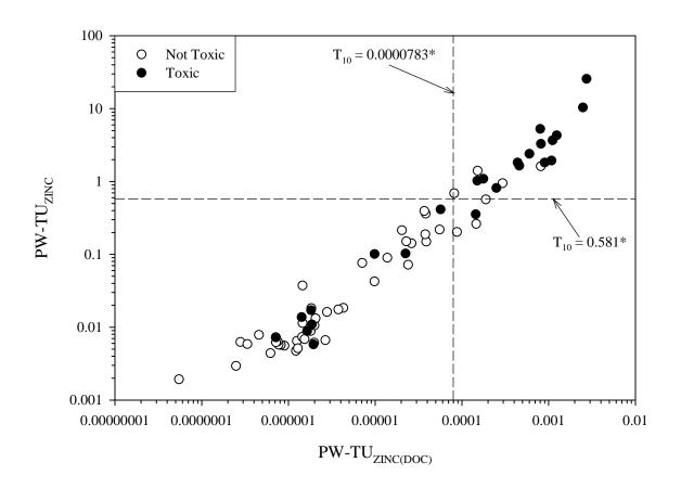
Figure A4-18. Scatter plot showing the relationship between pore-water zinc concentrations normalized to dissolved organic carbon (PW-TU<sub>ZINC(DOC)</sub>) and pore-water zinc concentrations (PW-TU<sub>ZINC</sub>), showing samples that were designated as toxic or not toxic based on the biomass of midges (*Chironomus dilutus*) in 10-d exposures to sediment samples from the Tri-State Mining District.
