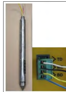
Figure 5.2: EC Wire Connections
