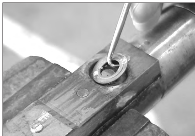
Figure 6.2 Remove and discard the copper washer.
