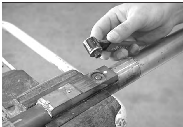
Figure 6.1 Unthread the membrane from the probe block.
