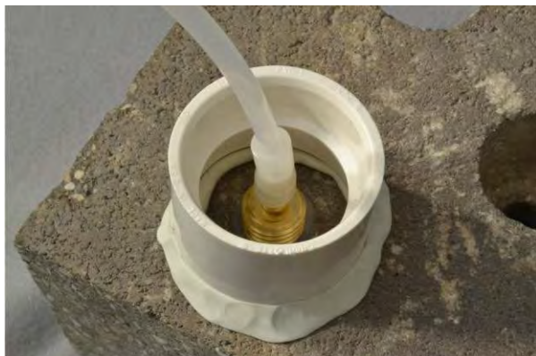
Figure 6. Water dam used for leak detection.
