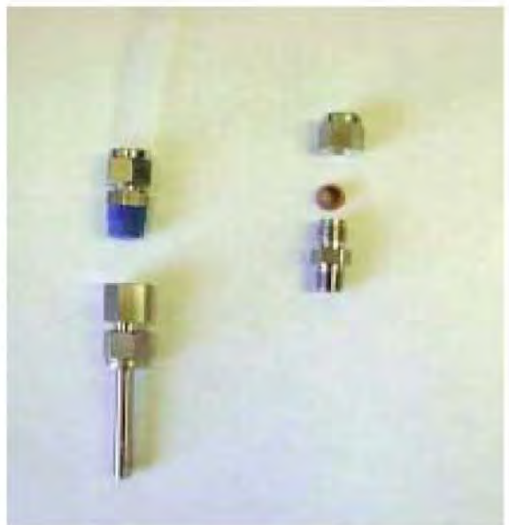
Figure 4. Stainless steel sub-slab vapor probe components
