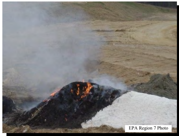
BIODIESEL FILTER MEDIA SPONTANEOUSLY COMBUSTING
